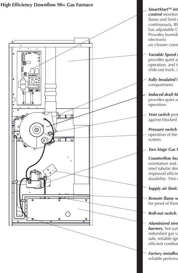
SmartStart™ integrated **control** monitors the burner flame and limit circuit continuously. Blower timing has adjustable OFF settings. Provides humidifier and air cleaner connections.
