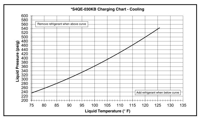
Figure 3. Charging Chart for 2.5 Ton Units S4QE-030KB Series (TXV Matches)
