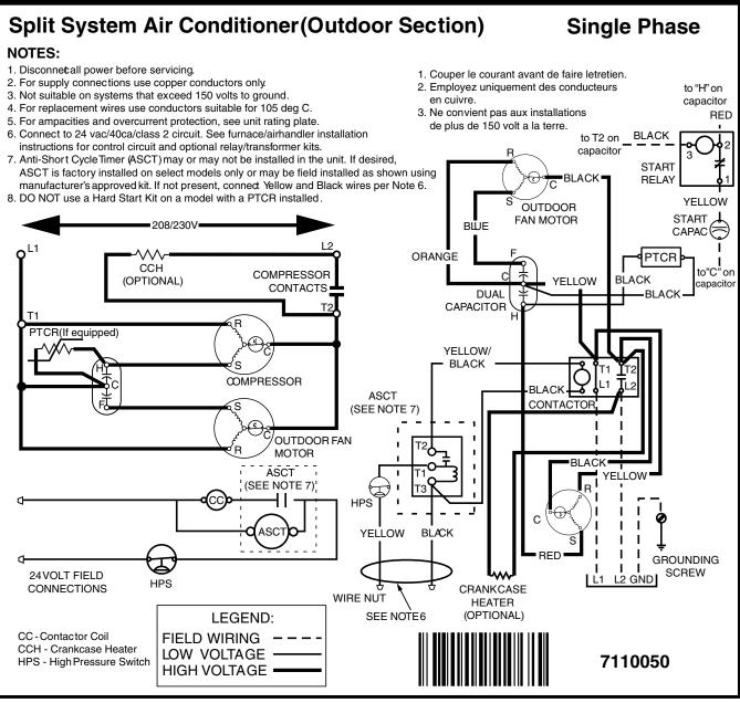
Figure 7. W.D. for 2 & 2.5 Ton Models
