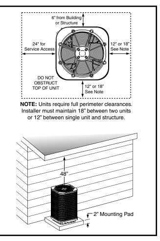
Figure 1. Clearance Requirements
