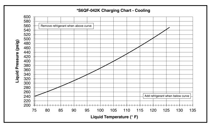
Figure 5. Charging Chart for 3.5 Ton Units S6QF-042K Series (TXV Matches)
