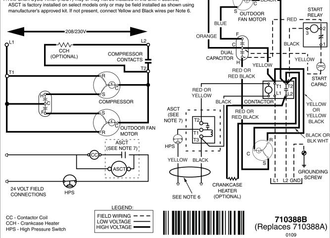
Figure 8. W.D. for 3 & 3.5 Ton Models
