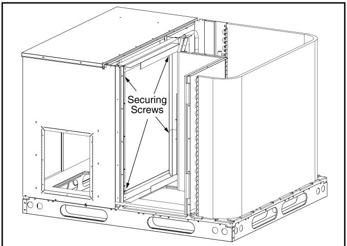
Figure 2. Internal Filter Rack Location
