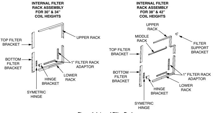
Figure 1. Internal Filter Rack
