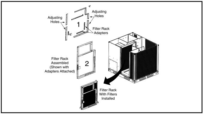
Figure 4. Internal Filter Rack Assembly for 24" Fan Orifice
