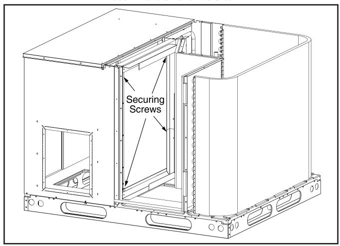
Figure 2. Internal Filter Rack Location
