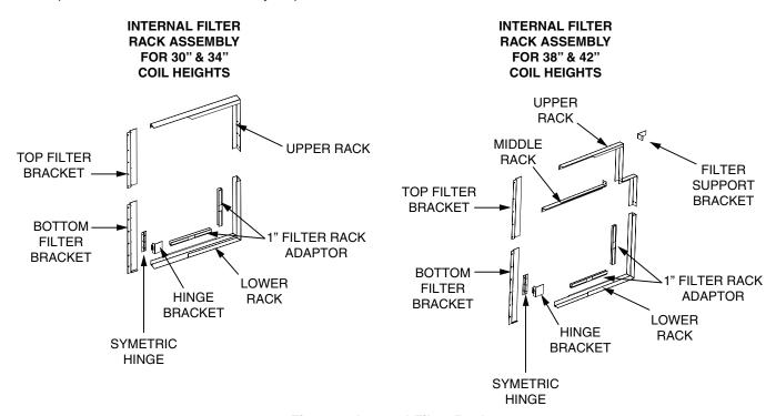
Figure 1. Internal Filter Rack
