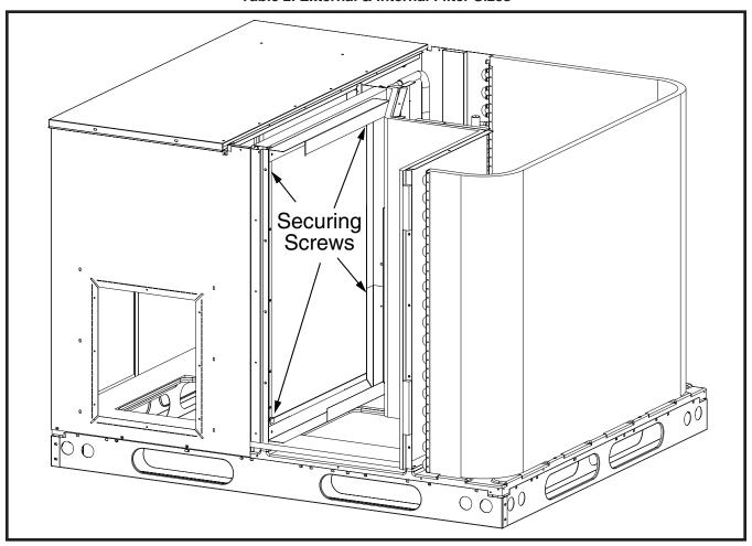
Figure 2. Internal Filter Rack Location
