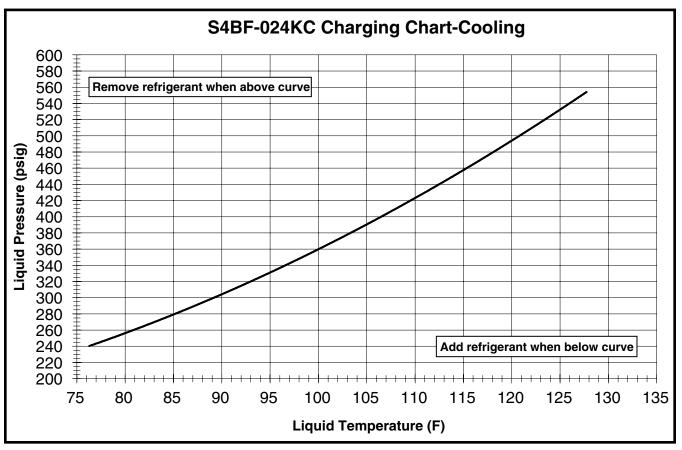
Figure 4. Charging Chart for 2 Ton Models
