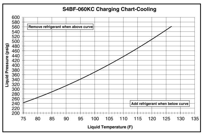
Figure 7. Charging Chart for 5 Ton Models
