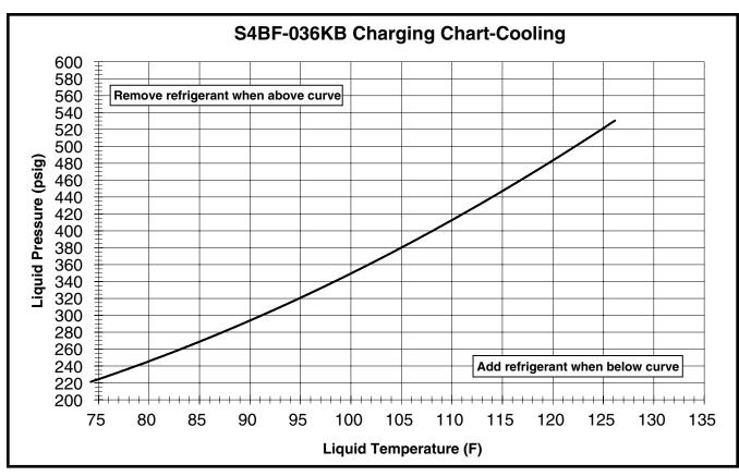
Figure 5. Charging Chart for 3 Ton Models
