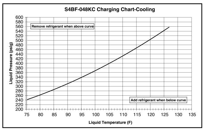
Figure 6. Charging Chart for 4 Ton Models
