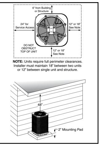
Figure 1. Clearance Requirements
