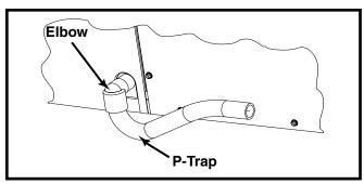
Figure 6. Drain Trap
