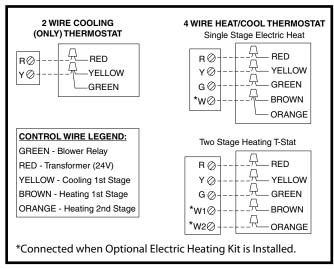
Figure 8. Low Voltage Connections
