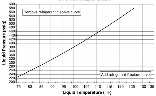
Figure 12. Charging Chart for 5 Ton Units (X60K Model)
