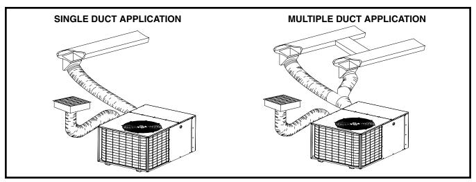
Figure 2. Single & Multiple Duct Applications
