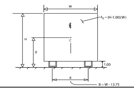
Figure 2: Calculate Wind Force
