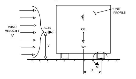
Figure 3: Calculate Lifting Force
