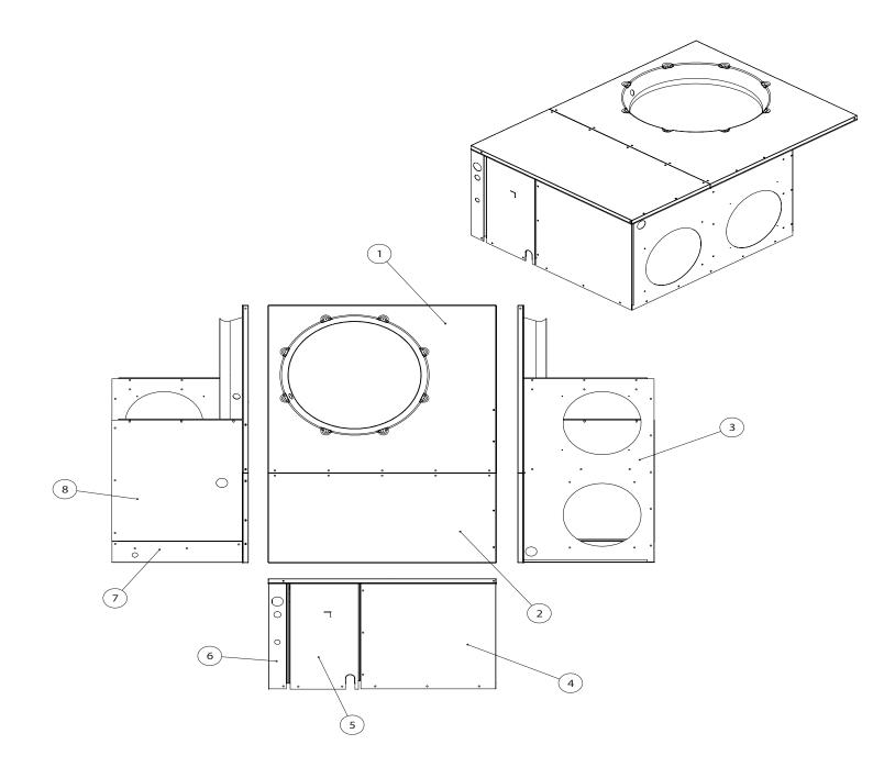
Figure 5. Panel Layout Single Package Unit
