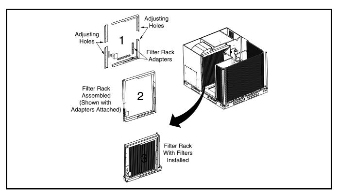
Figure 3. Internal Filter Rack Assembly for 20" Fan Orifice
