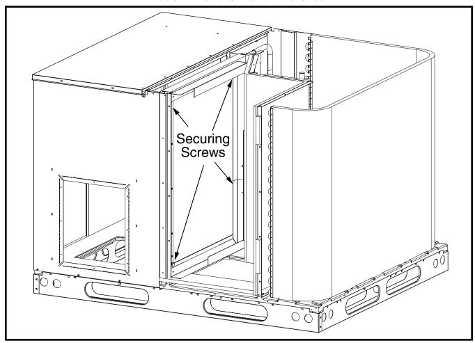
Figure 2. Internal Filter Rack Location
