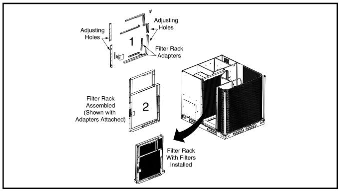
Figure 4. Internal Filter Rack Assembly for 24" Fan Orifice
