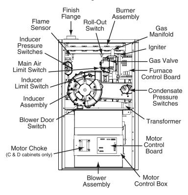
\*TC 95.1% Upflow / Horizontal Gas Furnace & \*TE 96% Gas Furnace (Upflow only)
