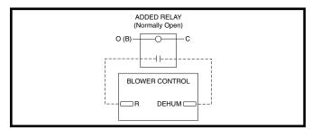
Figure 24. DEHUM Wiring Configuration without Humidistat
