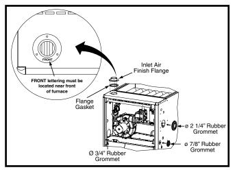
Figure 14. Finish Flange & Rubber Grommets
