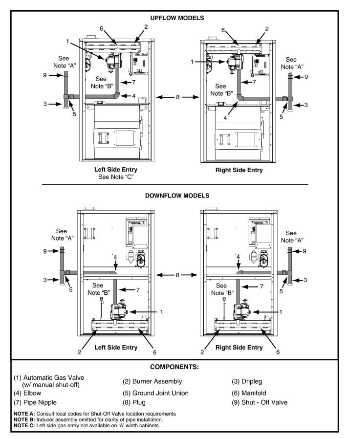
Figure 18. Typical Gas Connections
