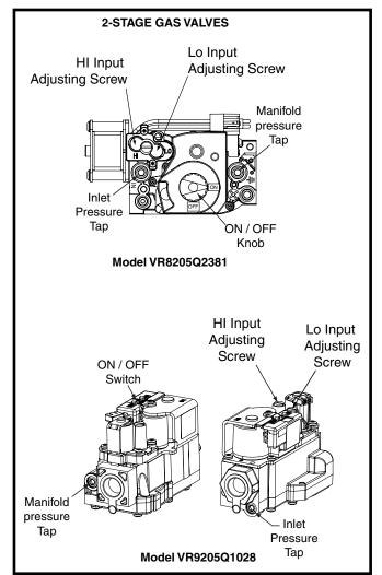
Figure 25. HI & LO Input Adjusting Screws
