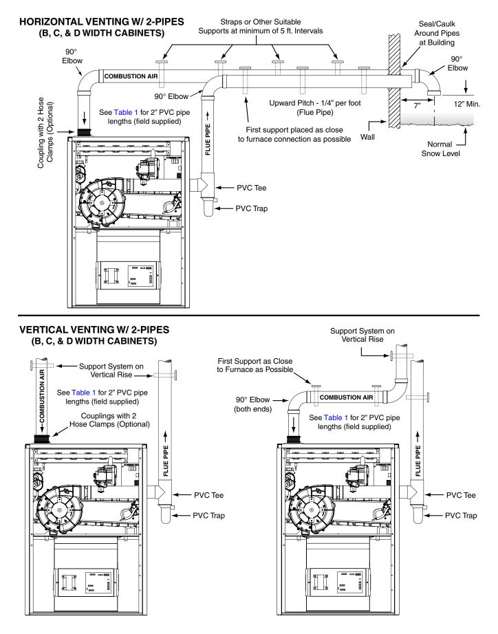
Figure 34. Horizontal & Vertical Venting (B, C, & D Width Cabinets)
