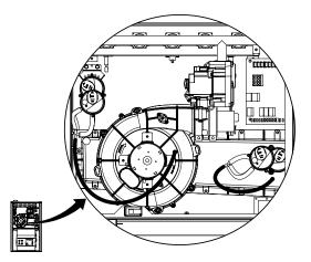
Figure 12. Pressure Switch Tubing for \*TE Upflow Furnaces
