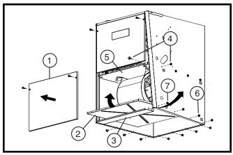
Figure 17. Alternate Removal Method
