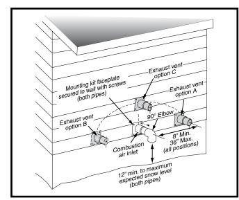
Figure 7. Inlet & Exhaust Pipe Clearances
