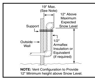
Figure 9. Alternate Horizontal Vent Installation
