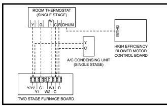
Figure 20. Wiring Configuration 1
