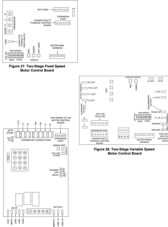
Figure 29. Two-Stage Furnace Control Board
