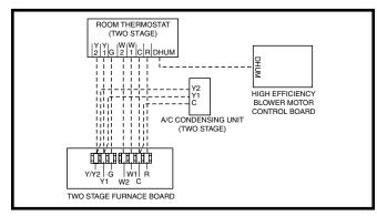
Figure 22. Wiring Configuration 3
