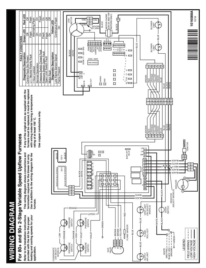
Figure 32. Wiring Diagram for Two-Stage, Variable Speed Upflow Furnaces
