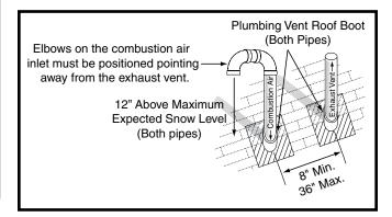
Figure 10. Vertical Vent Termination
