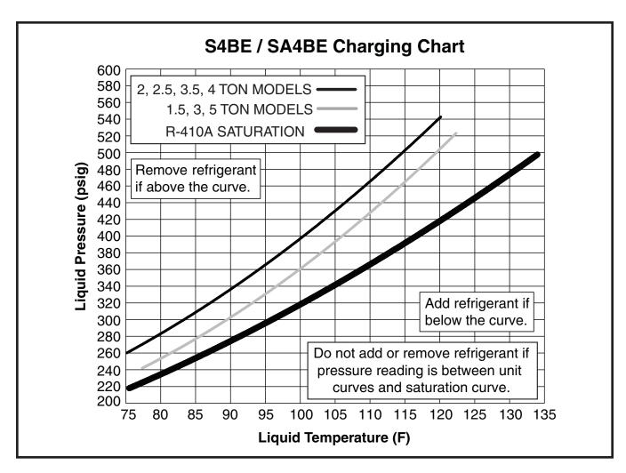
Figure 3. Charging Chart for 2 - 5 Ton Units
