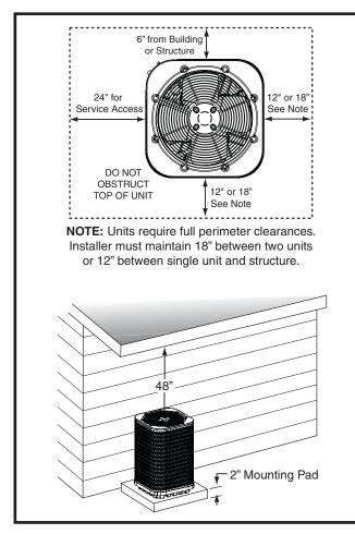
Figure 1. Clearance Requirements
