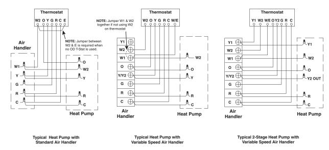
Figure 9. Typical Thermostat Connections
