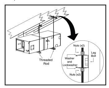
Figure 5. Unit Horizontally Suspended
