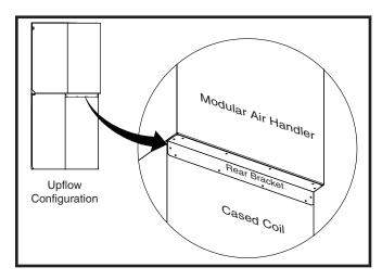
Figure 2. Rear Bracket Installation - (Upflow Only)
