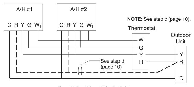
Figure 10. Low Voltage Wiring For Twinning
