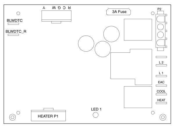
Figure 11. Single Stage Control Board (MB7BM Models)
