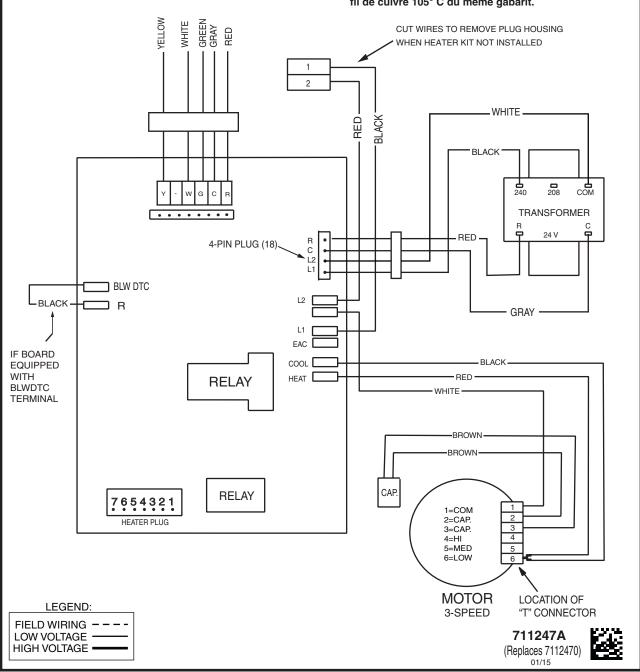
Figure 15. MB7BM Wiring Diagram
