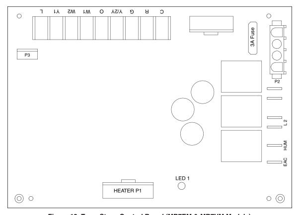
Figure 12. Two - Stage Control Board (MB7EM & MB7VM Models)
