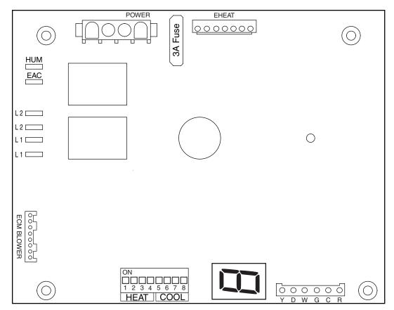
Figure 13. Fixed Speed Motor Control Board (MB7EM Models)
