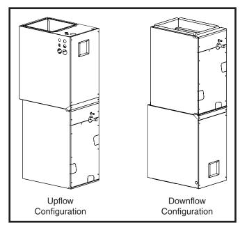
Figure 1. Upflow & Downflow Installation
