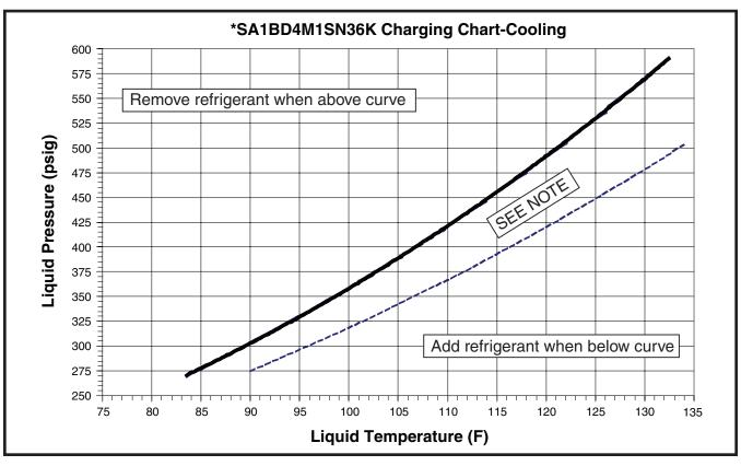
Figure 8. Charging Chart for 3 Ton Models (TXV Matches)
