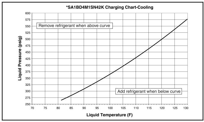
Figure 9. Charging Chart for 3.5 Ton Models (TXV Matches)
