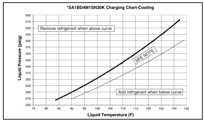
Figure 7. Charging Chart for 2.5 Ton Models (TXV Matches)
