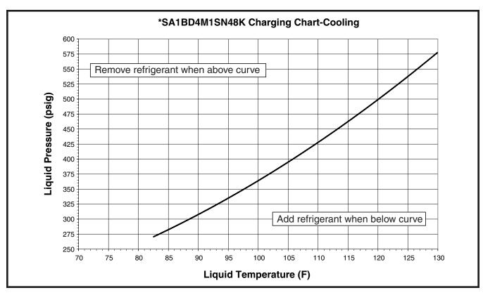
Figure 10. Charging Chart for 4 Ton Models (TXV Matches)
