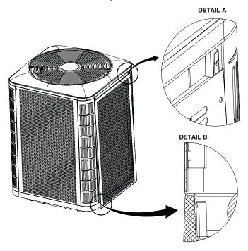
Figure 4. Panel Installation
