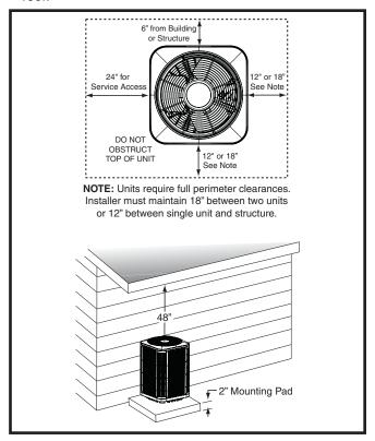
**Figure 1. Clearance Requirements**
