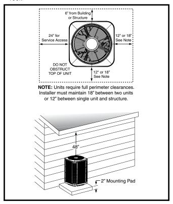
**Figure 1. Clearance Requirements**
