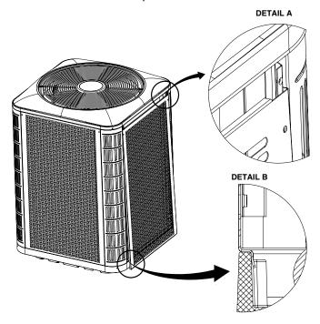
Figure 4. Panel Installation
