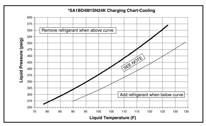
Figure 6. Charging Chart for 2 Ton Models (TXV Matches)
