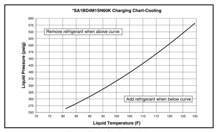
Figure 11. Charging Chart for 5 Ton Models (TXV Matches)
