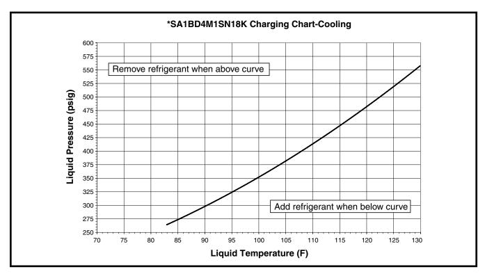
Figure 5. Charging Chart for 1.5 Ton Models (TXV Matches)
