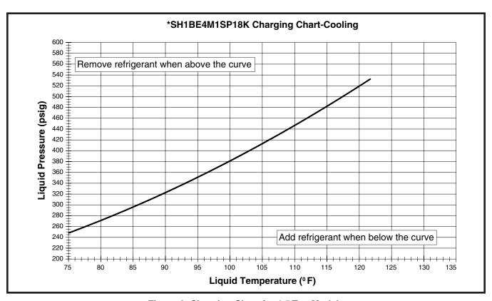
Figure 8. Charging Chart for 1.5 Ton Models (TXV Matches)
