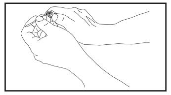
Figure 3. Removal of Orifice
