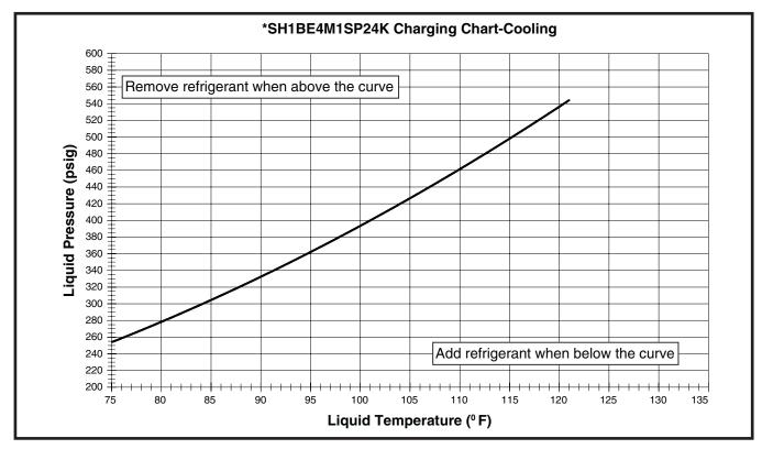
Figure 9. Charging Chart for 2 Ton Models (TXV Matches)
