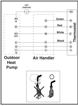
Figure 4. Typical Thermostat Connections
