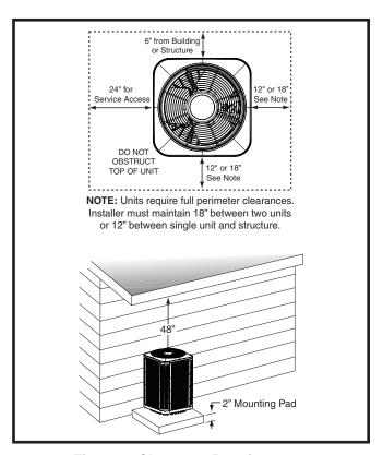
Figure 1. Clearance Requirements
