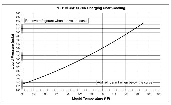
Figure 10. Charging Chart for 2.5 Ton Models (TXV Matches)
