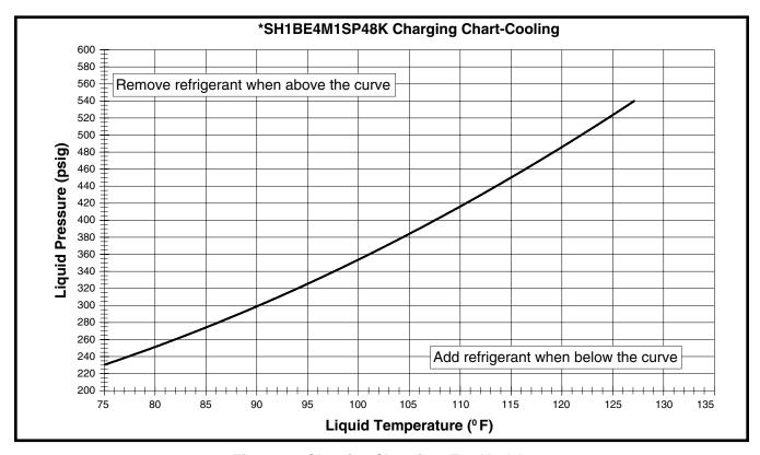
Figure 13. Charging Chart for 4 Ton Models (TXV Matches)
