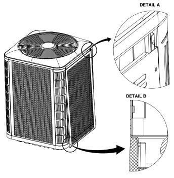
Figure 7. Panel Installation
