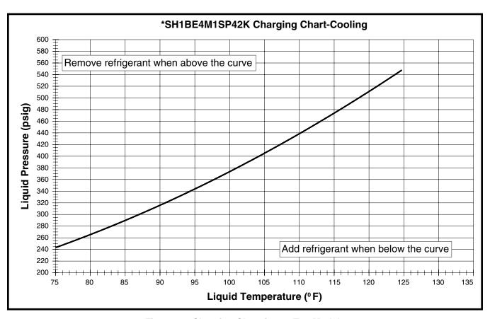
Figure 12. Charging Chart for 3.5 Ton Models (TXV Matches)
