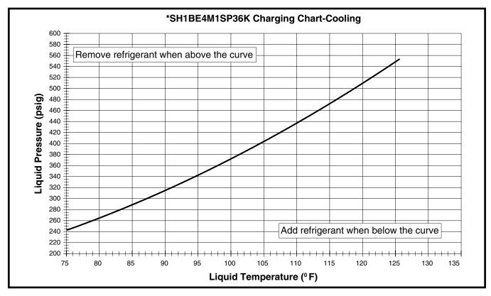
Figure 11. Charging Chart for 3 Ton Models (TXV Matches)
