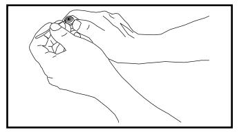
Figure 3. Removal of Orifice
