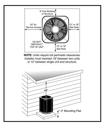
Figure 1. Clearance Requirements
