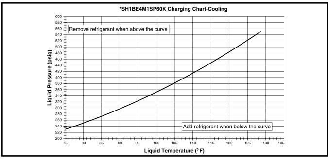
Figure 14. Charging Chart for 5 Ton Models (TXV Matches)
