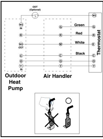
Figure 4. Typical Thermostat Connections
