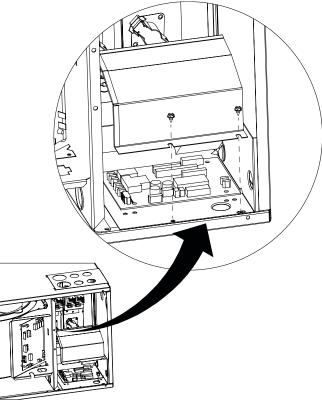
Figure 1. Installation of Drip Guard
