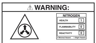
The coil in the air handler is factory shipped with a nitrogen charge. Avoid direct face exposure or contact with valve when gas is escaping. Always ensure adequate ventilation is present during the depressurization process. Address any uncertainties before proceeding. Failure to comply with this warning could result in equipment damage, personal injury, or death.
