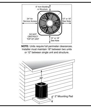
**Figure 1. Clearance Requirements**
