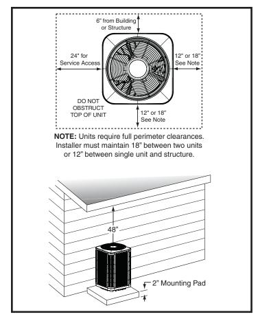
**Figure 1. Clearance Requirements**
