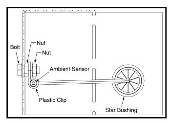
Figure 6. Ambient Sensor Mounting
