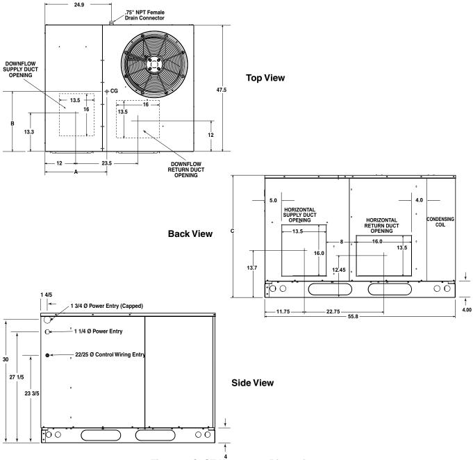
Figure 7. Q6SE Heat pump Dimensions
