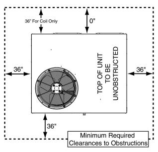
**Figure 2. Clearance Requirements**
