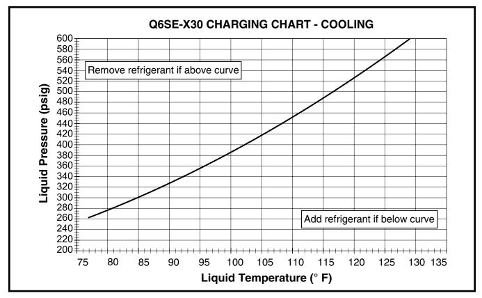
Figure 11. Charging Chart for 2.5 Ton Units
