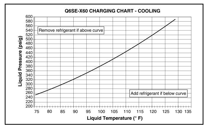
Figure 15. Charging Chart for 5 Ton Units
