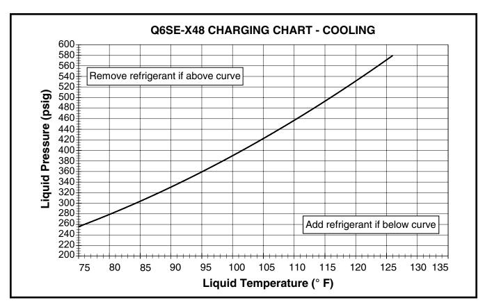
Figure 14. Charging Chart for 4 Ton Units
