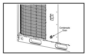
Figure 5. Condensate Drain Location
