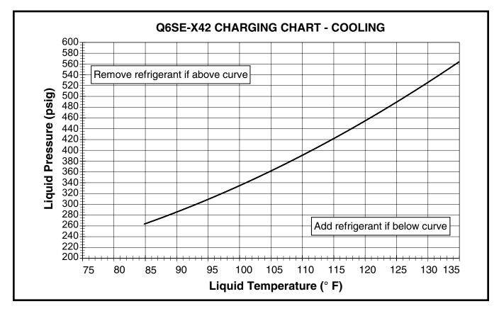
Figure 13. Charging Chart for 3.5 Ton Units
