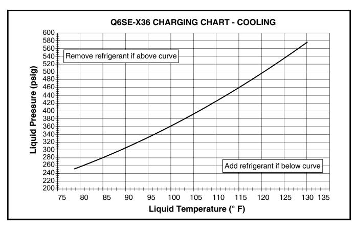
Figure 12. Charging Chart for 3 Ton Units
