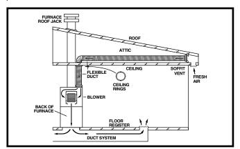
Figure 5. General Install Setup
