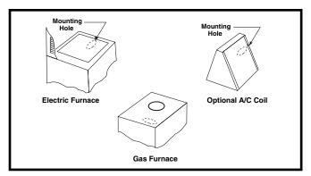
Figure 1. Plastic Inlet Fitting Location
