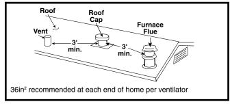
Figure 4. Roof Spacing
