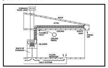
Figure 5. General Install Setup
