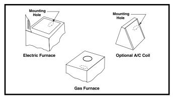
Figure 1. Plastic Inlet Fitting Location
