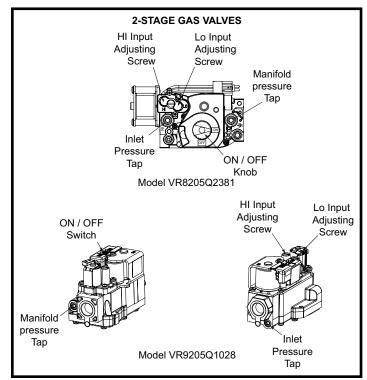
Figure 8. HI & LO Input Adjusting Screws
