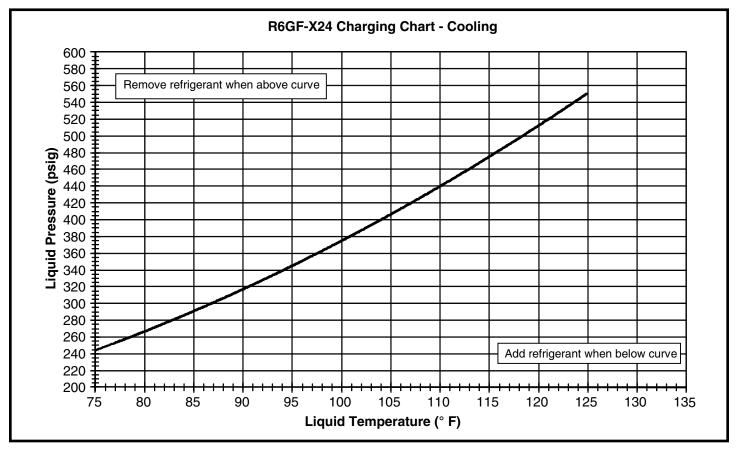
Figure 15. Charging Chart for 2 Ton Units
