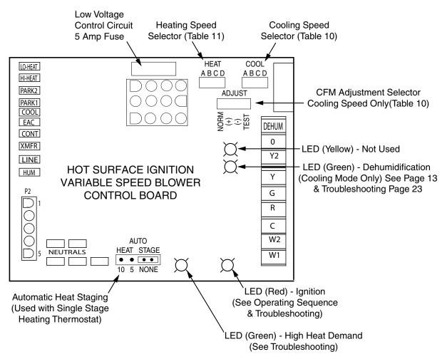
Figure 12. Two-Stage, Hot Surface Ignition & Blower Control Board
