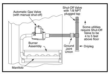
Figure 7. Typical Gas Hookup - Right Side Entry
