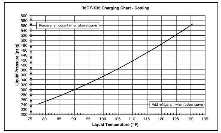
Figure 16. Charging Chart for 3 Ton Units
