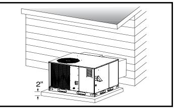
Figure 3. Ground Level Installation
