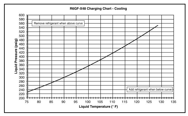
Figure 17. Charging Chart for 4 Ton Units
