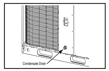
Figure 5. Condensate Drain Location
