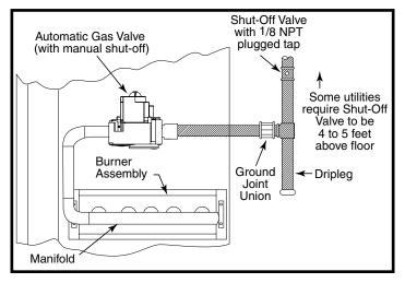
Figure 8. Typical Gas Hookup - Right Side Entry
