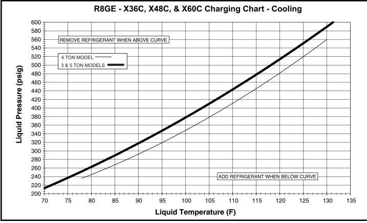
Figure 13. Charging Chart for 3 Ton Units
