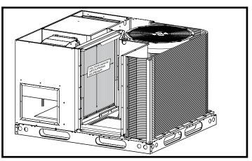
Figure 6. Internal Filter Rack Location
