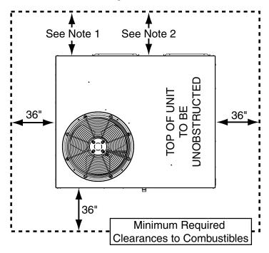
**NOTE 1:** 6" When coil is present on duct side. **NOTE 2:** 1" When no coil is present on duct side.
