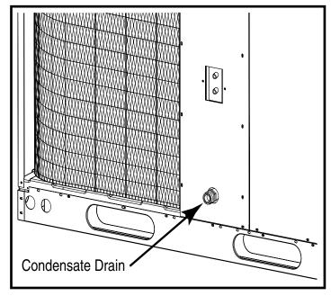
Figure 5. Condensate Drain Location
