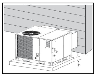
Figure 3. Ground Level Installation
