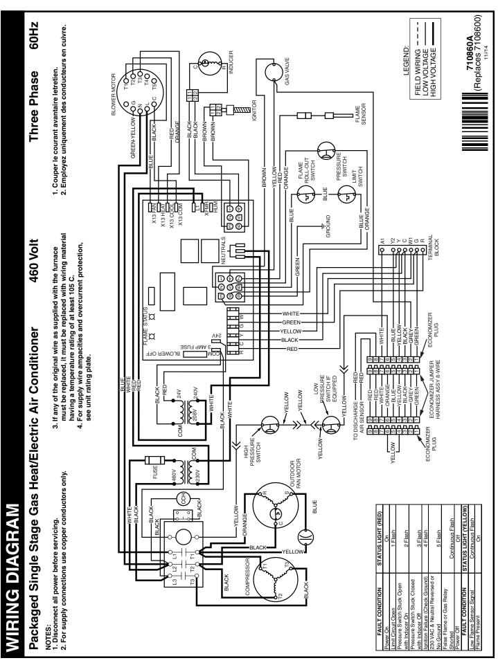
Figure 12. Wiring Diagram for 460V / 3 Phase / 60 Hz Unit
