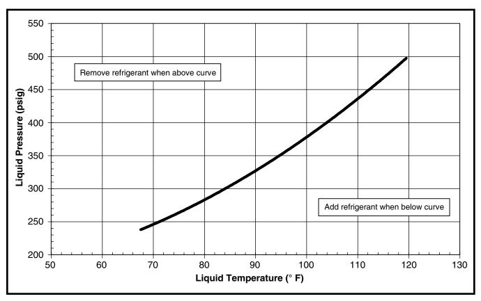
Figure 21. Charging Chart for 4 Ton Units
