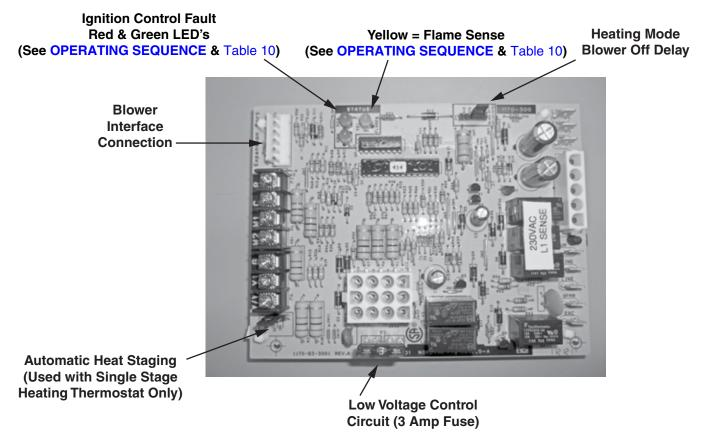
Figure 12. Two-Stage, Hot Surface Ignition & Blower Control Board
