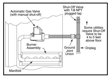
Figure 7. Typical Gas Hookup - Right Side Entry
