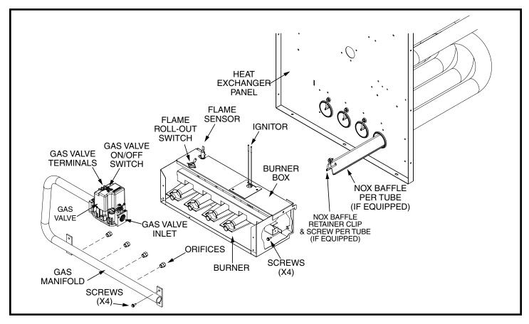
Figure 8. Burner & Manifold Assembly
