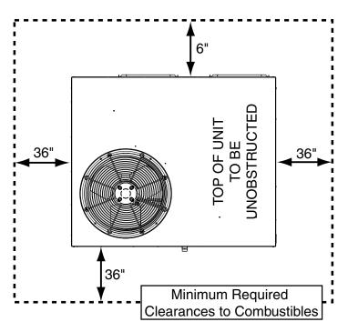
Figure 1. Clearance Requirements
