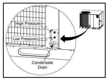
Figure 5. Condensate Drain & Service Ports
