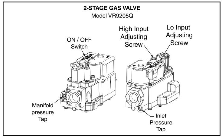
Figure 9. HI & LO Input Adjusting Screws
