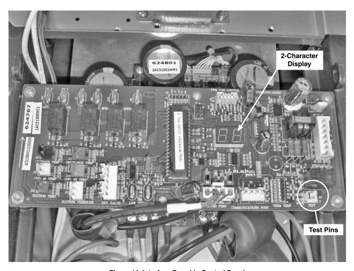
Figure 14. Interface Board in Control Panel
