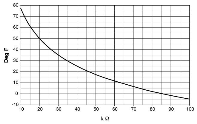
**Figure 23. Temperature Sensor Resistance Charts**
