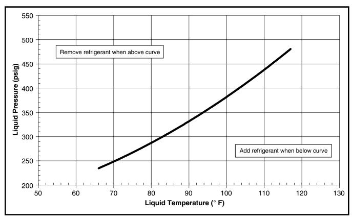
Figure 20. Charging Chart for 3 Ton Units
