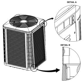
Figure 4. Panel Installation
