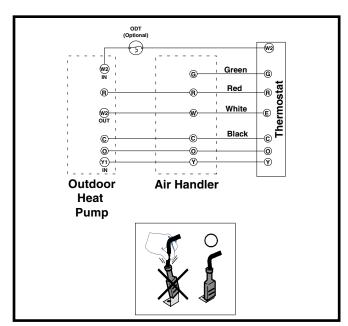
Figure 2. Typical Thermostat Connections
