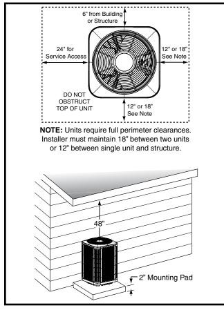
Figure 1. Clearance Requirements
