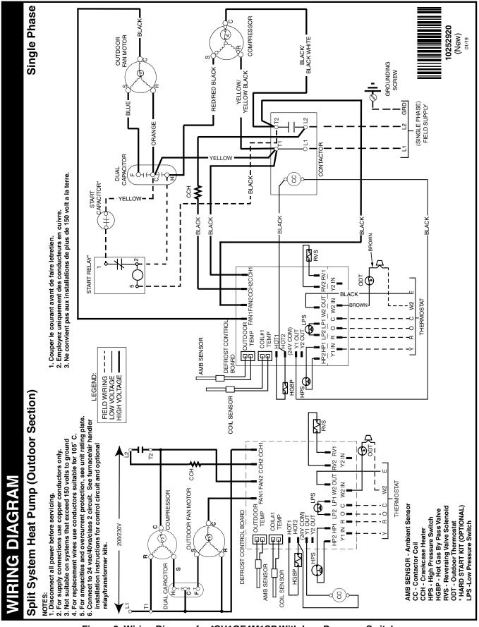
Figure 8. Wiring Diagram for \*SH1QE4M1SP With Low Pressure Switch
