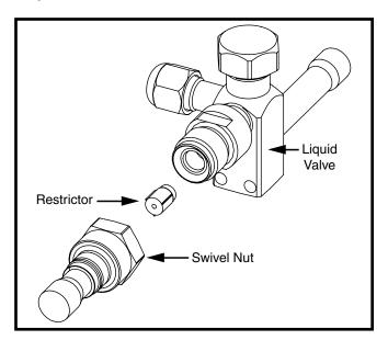
Figure 2. Liquid Valve, Restrictor, & Swivel Nut Adapter
