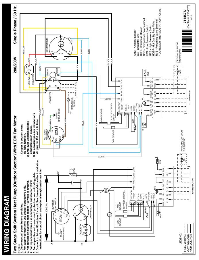
Figure 12. Wiring Diagram for \*SH(1,2)BF4M2SX (5 Ton Units)
