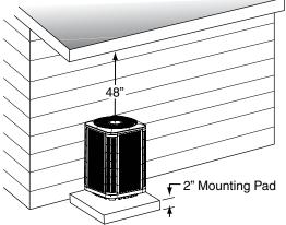
**Figure 1. Clearance Requirements**
