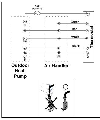
Figure 4. Thermostat Connections for SH1BF4M1SP 2 - 4 Ton Units
