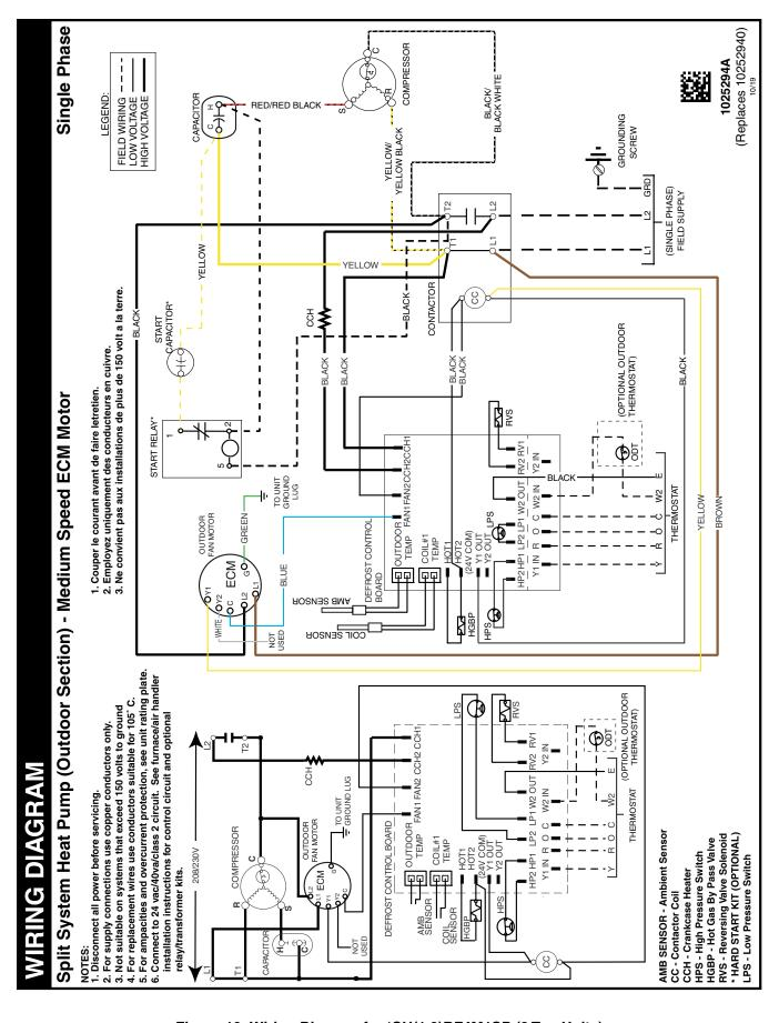
Figure 10. Wiring Diagram for \*SH(1,2)BF4M1SP (3 Ton Units)
