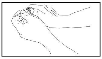
Figure 3. Removal of Orifice
