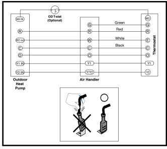
Figure 5. Thermostat Connections for SH1BF4M2SX 5-Ton Units
