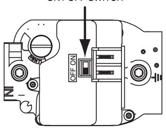
Figure 2. Single Stage Gas Valve
