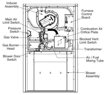
Figure 1. G8SA Furnace Components
