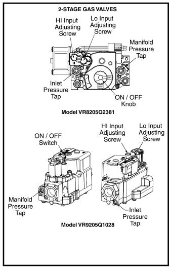
Figure 20. HI & LO Input Adjusting Screws
