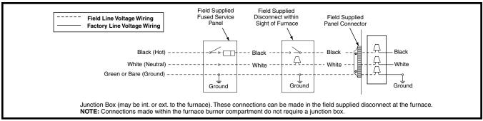
Figure 14. Line Voltage Field Wiring
