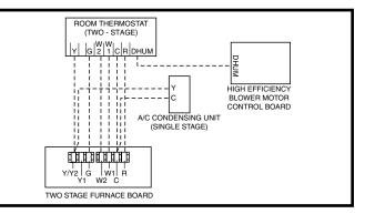
Figure 16. Wiring Configuration 2
