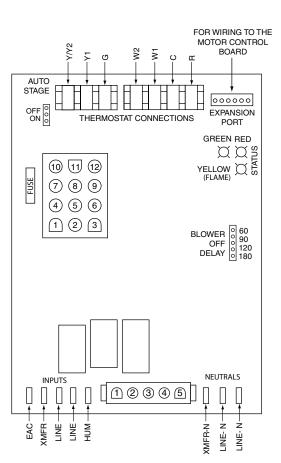
Figure 24. Two-Stage Furnace Control Board
