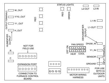
Figure 23. Two-Stage Variable Speed Motor Control Board
