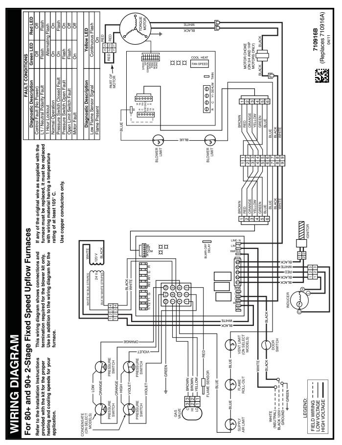
Figure 25. Wiring Diagram for Two-Stage, Fixed Speed Upflow Furnaces
