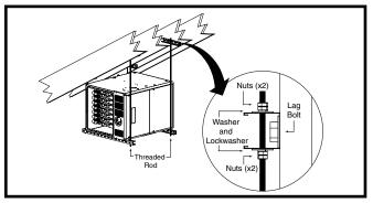
Figure 8. \*TA Horizontally Suspended in Attic
