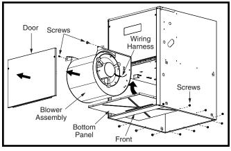
Figure 11. Bottom Panel Removal
