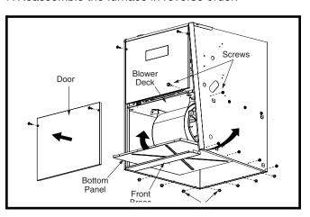
Figure 12. Alternate Removal Method
