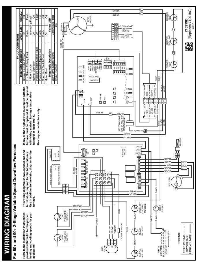
Figure 28. Wiring Diagram for Two-Stage, Variable Speed Downflow Furnaces
