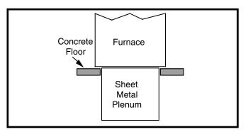
Figure 9. Furnace on a Concrete Slab
