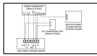
Figure 15. Wiring Configuration 1
