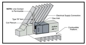
Figure 7. \*TA Horizontally Installed on a Platform
