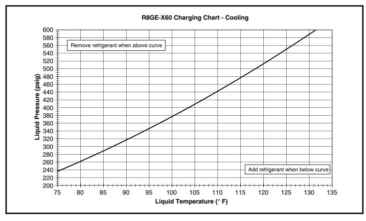
Figure 12. Charging Chart for 5 Ton Models
