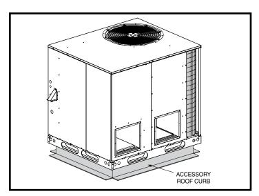
Figure 3. Roof Top Installation
