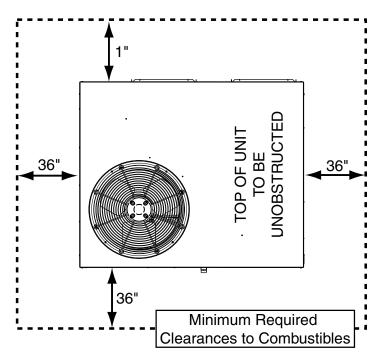
Figure 1. Clearance Requirements
