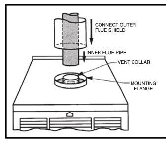
Figure 22. Combustion Air Pipe Connection
