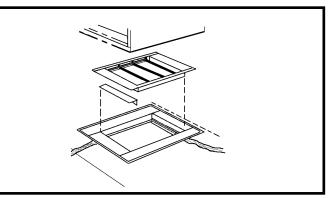
Figure 30. Without Coil Cavity Damper
