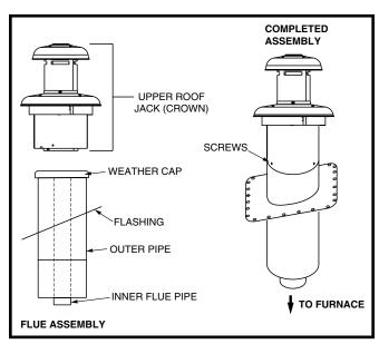
Figure 23. Roof Jack Crown
