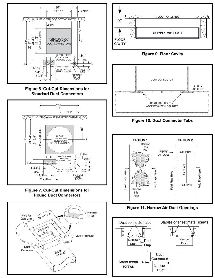
Figure 8. Standard Duct Connector Installed
