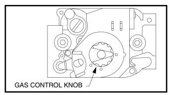
Figure 28. Direct Ignition Gas Valve - Honeywell
