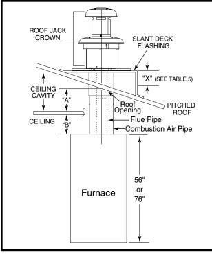
Figure 16. Ceiling Cavity Depth
