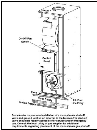
Figure 26. Typical Gas Piping
