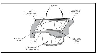
Figure 13. Round Duct Connector Installed
