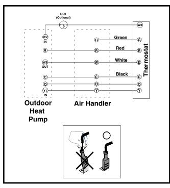
Figure 4. Typical Thermostat Connections
