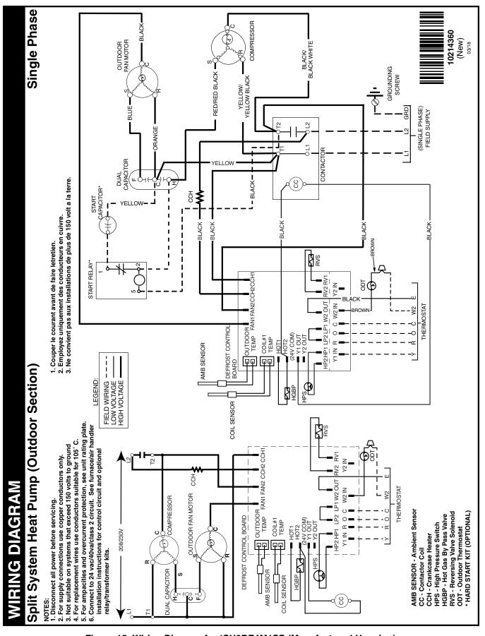
Figure 15. Wiring Diagram for \*SH2BE4M1SP (Manufactured Housing)
