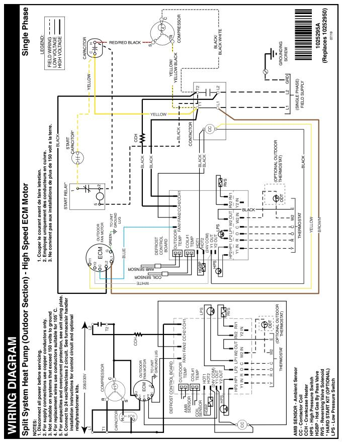
Figure 10. Wiring Diagram for \*SH(1,2)BE4M1SP60K (5 Ton) (with Low Pressure Switch)
