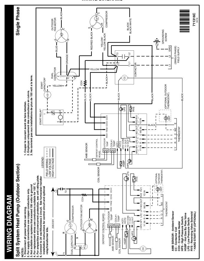
Figure 9. Wiring Diagram for \*SH(1,2)BE4M1SP (1.5 Ton - 4 Ton) (with Low Pressure Switch)
