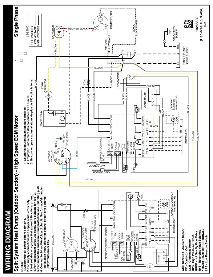
Figure 12. Wiring Diagram for \*SH1BE4M1SP60KA (5 Ton) (with CoreSense™ and Low Pressure Switch)
