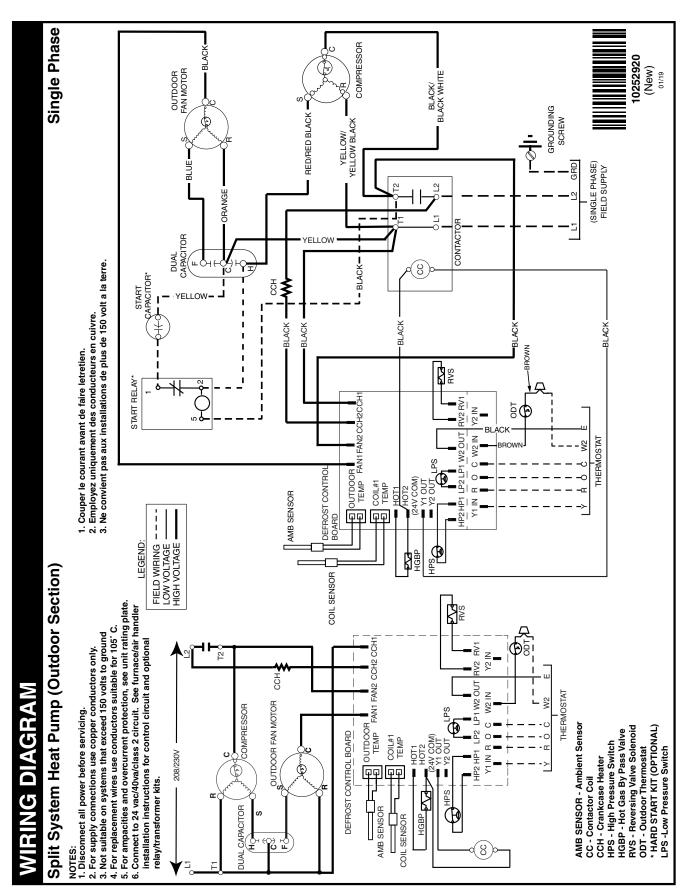
Figure 13. Wiring Diagram for \*SH1BE4M1SP with Low Pressure Switch (Manufactured Housing)
