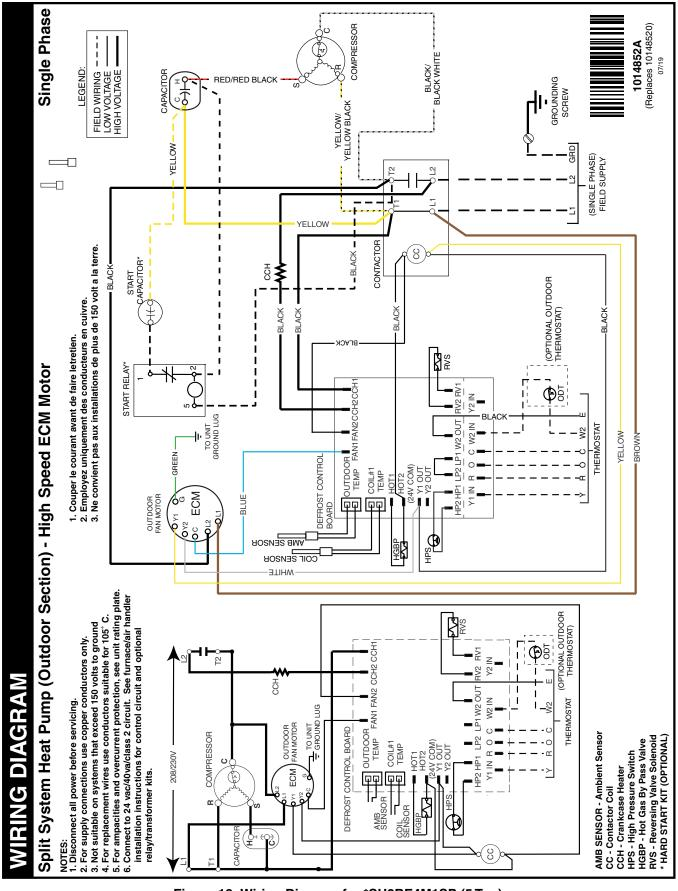
Figure 18. Wiring Diagram for \*SH2BE4M1SP (5 Ton) (Builder's Series)
