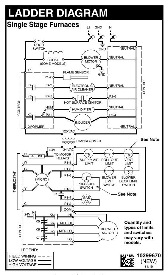
Figure 46. MG3P Ladder Diagram
