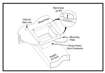
Figure 18. Screw-Down Duct Connector
