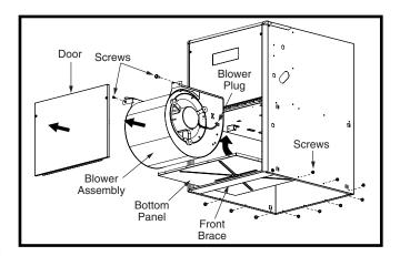
Figure 22. Bottom Panel Removal
