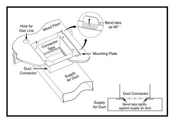
Figure 14. Duct Connector Installed
