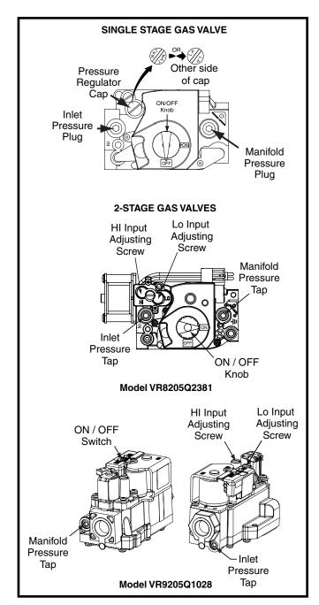
Figure 36. Gas Valve - Top View
