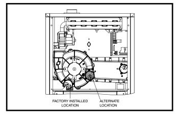
Figure 26. Alternate Pressure Switch Location
