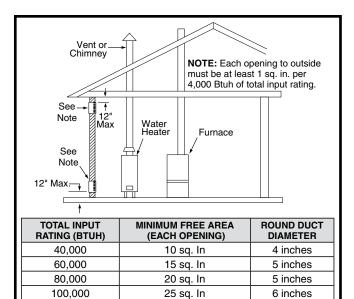
Figure 6. Combustion Air Drawn from Outside Through an Exterior Wall
