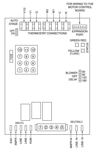
Figure 50. Two-Stage Furnace Control Board
