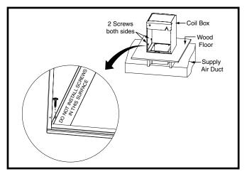
Figure 20. A/C Coil Box Installation
