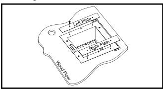
Figure 15. Duct Connector Side Plates
