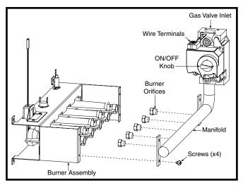
Figure 37. Burner & Manifold Assembly
