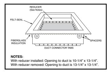
Figure 12. Duct Connector
