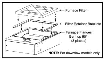
Figure 32. Filter Retainer Brackets
