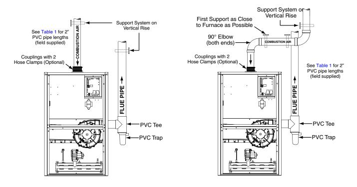
Figure 52. MG3S Horizontal & Vertical Venting
