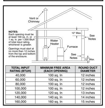
Figure 2. Combustion Air Drawn from Inside
