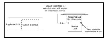
Figure 17. Narrow Air Ducts - Option 2
