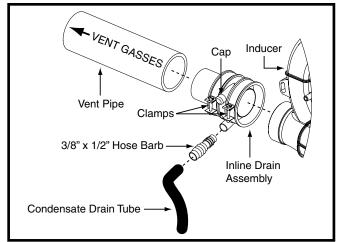
Figure 29. Inline Drain Assembly
