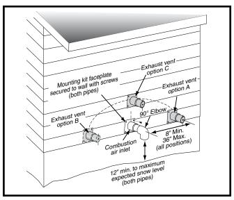
Figure 7. Inlet & Exhaust Pipe Clearances
