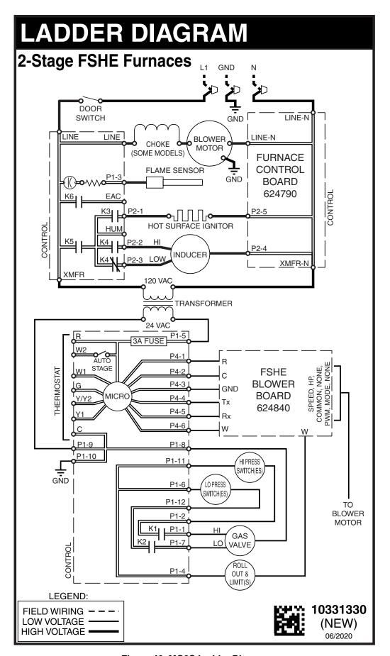
Figure 48. MG3S Ladder Diagram
