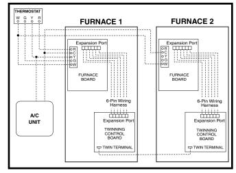
Figure 43. Single Stage Twinning
