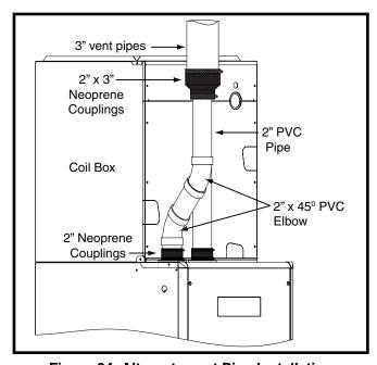
Figure 34. Alternate vent Pipe Installation
