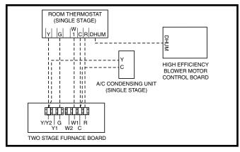
Figure 38. Wiring Configuration 1
