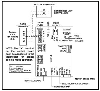
Figure 42. Low Voltage Field, Four-wire Heating / Cooling Applications
