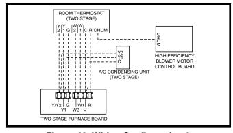
Figure 40. Wiring Configuration 3
