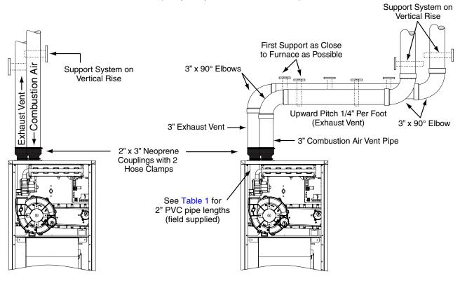
Figure 51. MG3P Horizontal & Vertical Venting
