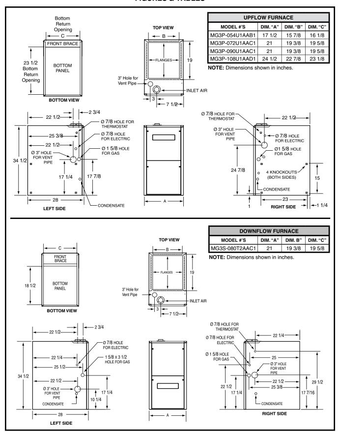
Figure 44. Furnace Dimensions
