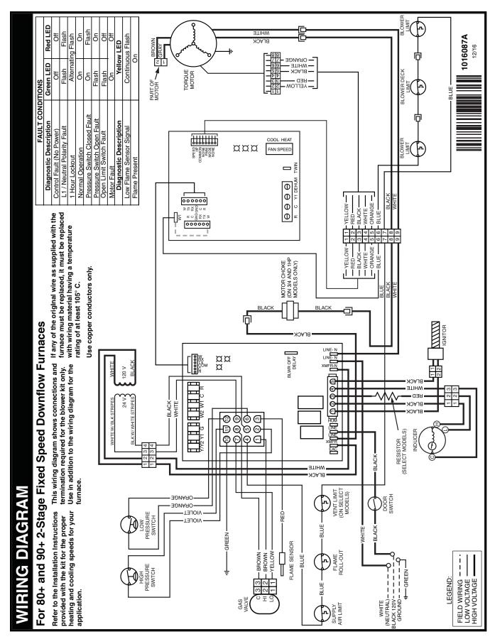
Figure 47. MG3S Wiring Diagram
