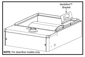
Figure 33. VentilAire™ Bracket
