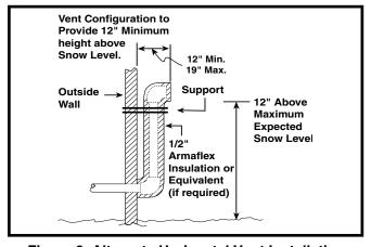
Figure 9. Alternate Horizontal Vent Installation
