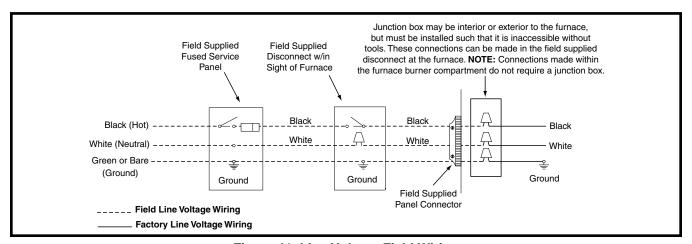
Figure 41. Line Voltage Field Wiring
