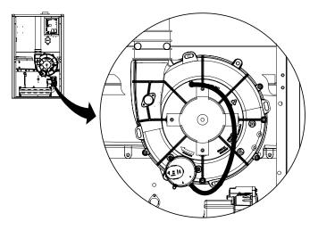
Figure 25. Pressure Switch Tubing for Downflow Furnaces (Model: MG3S-080)
