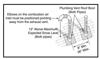
Figure 10. Vertical Vent Termination
