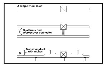
Figure 11. Typical Supply Duct System
