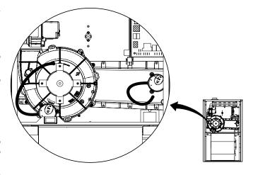
Figure 24. Pressure Switch Tubing for Upflow Furnaces (Models: MG3P-054 & MG3P-090)
