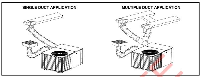
Figure 2. Single & Multiple Duct Applications
