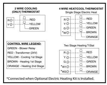
Figure 8. Low Voltage Connections
