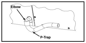
Figure 6. Drain Trap
