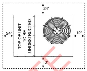
Figure 1. Minimum Unit Clearances
