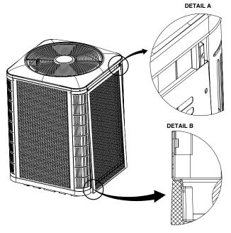
Figure 4. Panel Installation
