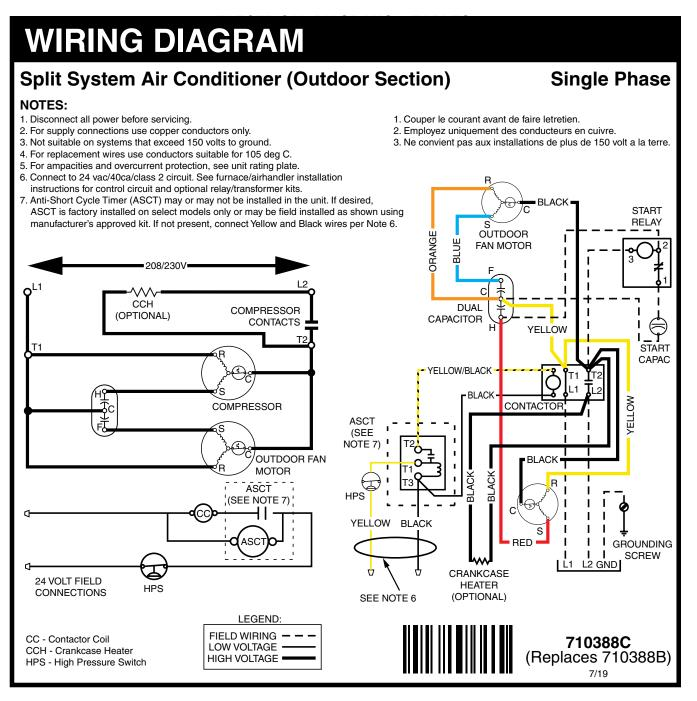
Figure 5. Wiring Diagram for \*SA(1,2)BD4M1SN (1.5, 2, 2.5, 3, 3.5, 4, & 5 Ton Units)
