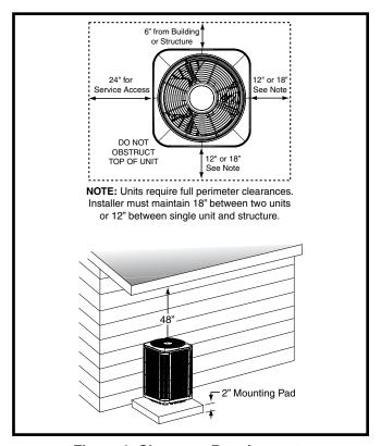
**Figure 1. Clearance Requirements**
