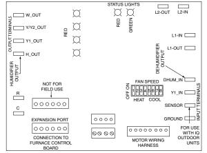
Figure 28. Two-Stage Variable Speed Motor Control Board
