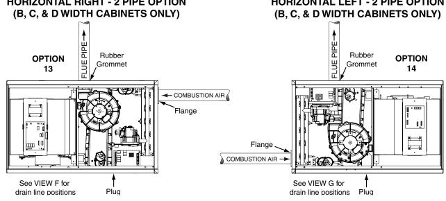
Figure 37. Horizontal Venting Options (B, C, & D Width Cabinets)
