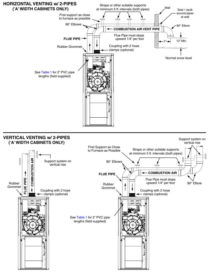
Figure 32. Horizontal & Vertical Venting (A Width Cabinets)
