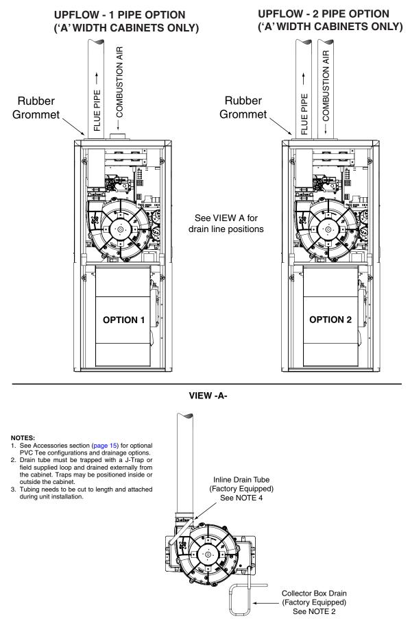
Figure 34. Upflow Venting Options (A Width Cabinets)
