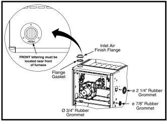
Figure 14. Finish Flange & Rubber Grommets
