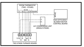
Figure 21. Wiring Configuration 2
