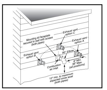
Figure 7. Inlet & Exhaust Pipe Clearances
