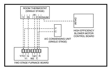
Figure 20. Wiring Configuration 1
