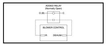
Figure 24. DEHUM Wiring Configuration without Humidistat
