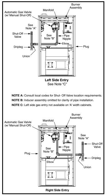
Figure 18. Typical Gas Connections
