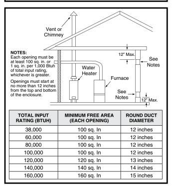
Figure 2. Combustion Air Drawn from Inside
