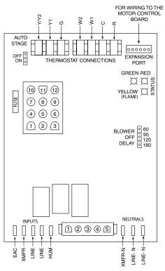
Figure 29. Two-Stage Furnace Control Board
