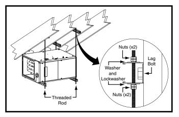
Figure 12. \*TC Horizontally Suspended in Attic
