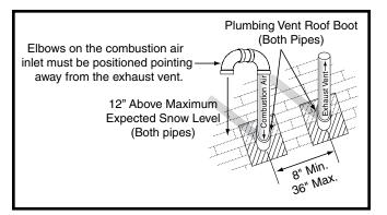
**Figure 10. Vertical Vent Termination**
