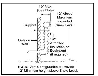
Figure 9. Alternate Horizontal Vent Installation
