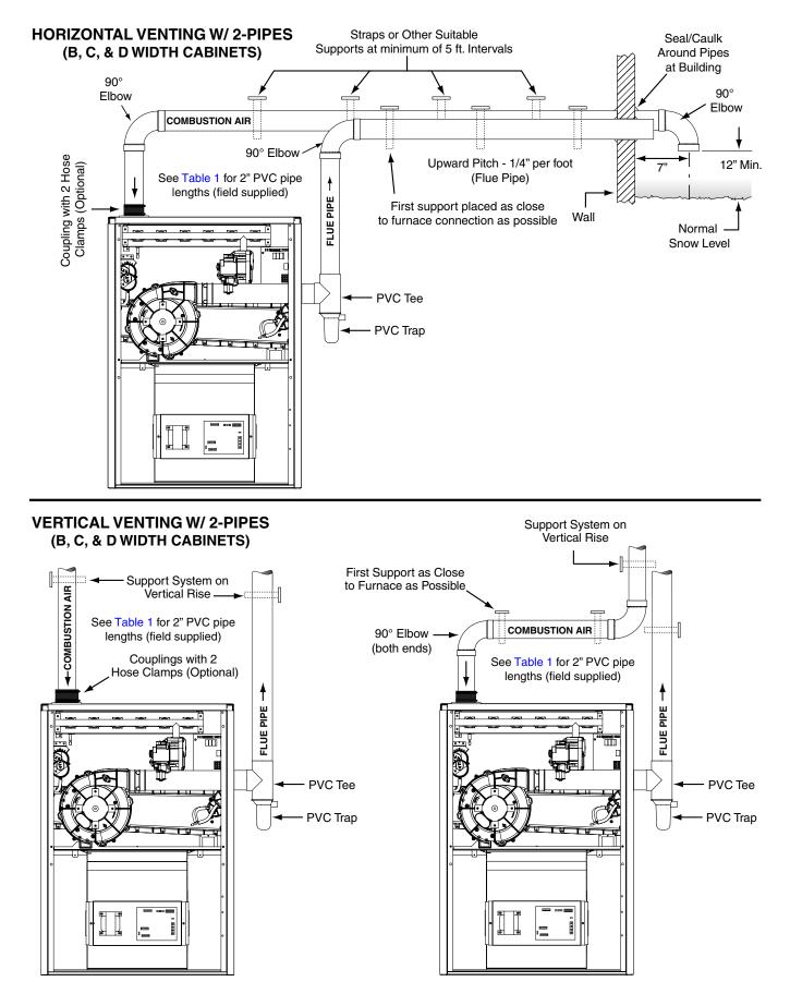
Figure 33. Horizontal & Vertical Venting (B, C, & D Width Cabinets)
