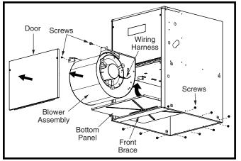
Figure 16. Bottom Panel Removal
