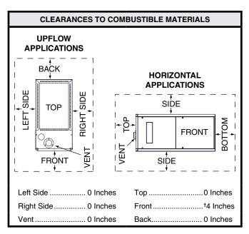
$\ensuremath{+}\xspace$  Allow 24 in. minimum clearance for servicing. Recommended clearance is 36 in.
