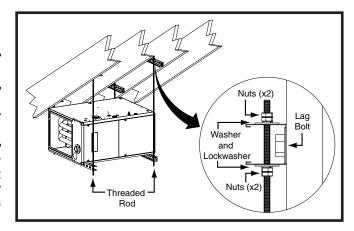
Figure 12. \*TC Horizontally Suspended in Attic
