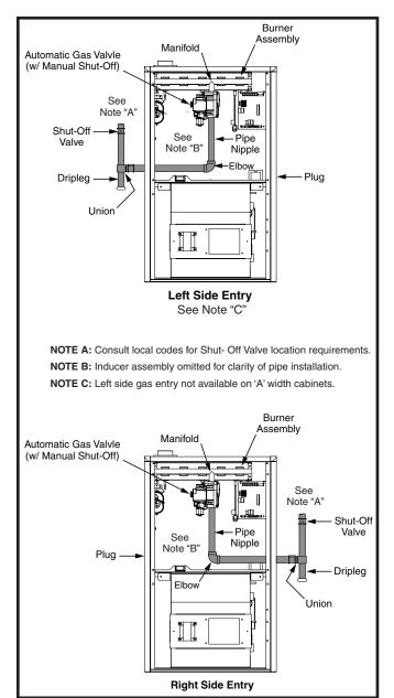
Figure 18. Typical Gas Connections
