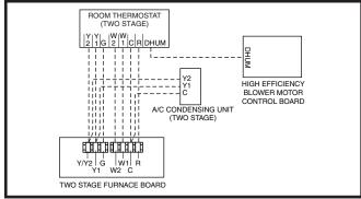
Figure 22. Wiring Configuration 3
