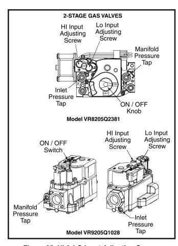
Figure 25. HI & LO Input Adjusting Screws
