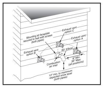
Figure 7. Inlet & Exhaust Pipe Clearances
