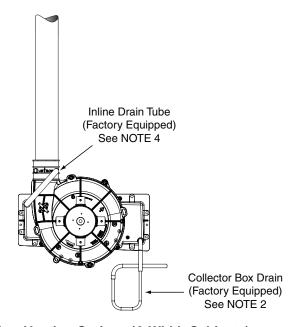
Figure 34. Upflow Venting Options (A Width Cabinets)
