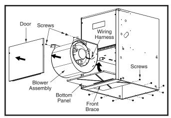
Figure 16. Bottom Panel Removal
