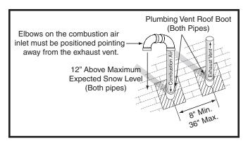
**Figure 10. Vertical Vent Termination**
