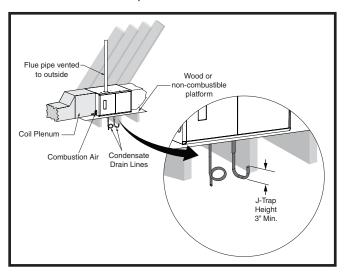
Figure 11. \*TC Horizontally Installed on a Platform
