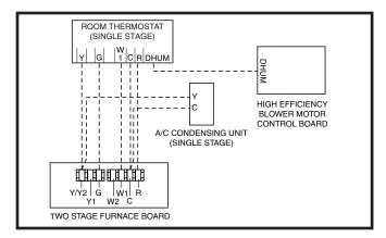
Figure 20. Wiring Configuration 1
