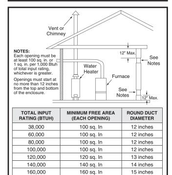
Figure 2. Combustion Air Drawn from Inside
