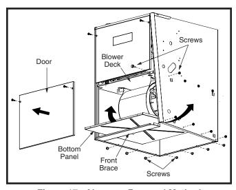
Figure 17. Alternate Removal Method
