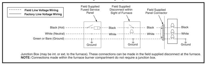
Figure 19. Line Voltage Field Wiring
