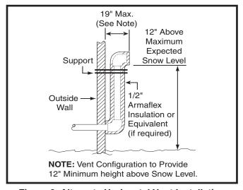
Figure 9. Alternate Horizontal Vent Installation
