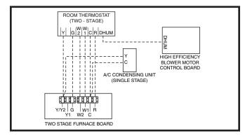
Figure 21. Wiring Configuration 2
