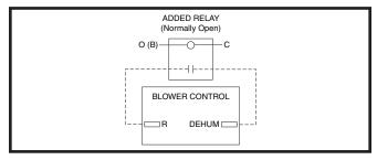
Figure 24. DEHUM Wiring Configuration without Humidistat
