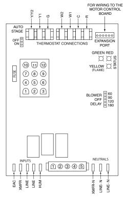
Figure 29. Two-Stage Furnace Control Board
