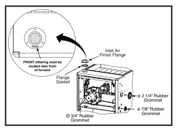
Figure 14. Finish Flange & Rubber Grommets
