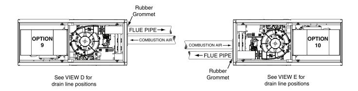
Figure 36. Horizontal Venting Options (A Width Cabinets)
