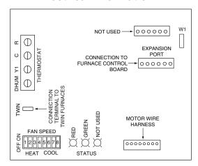
Figure 27. Two-Stage Fixed Speed Motor Control Board
