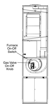
Figure 2. MG1 Gas Furnace Components
