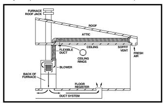
Figure 5. General Install Setup
