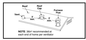
Figure 4. Roof Spacing
