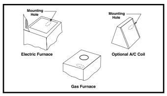
Figure 1. Plastic Inlet Fitting Location
