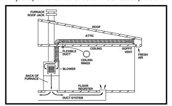
Figure 5. General Install Setup
