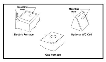
Figure 1. Plastic Inlet Fitting Location
