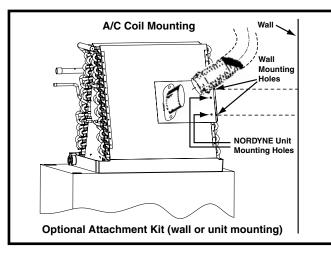
Figure 2. Downflow Electric Furnace with A/C
