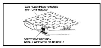
Figure 4. Installation Detail
