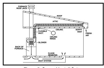
Figure 5. General Install Setup
