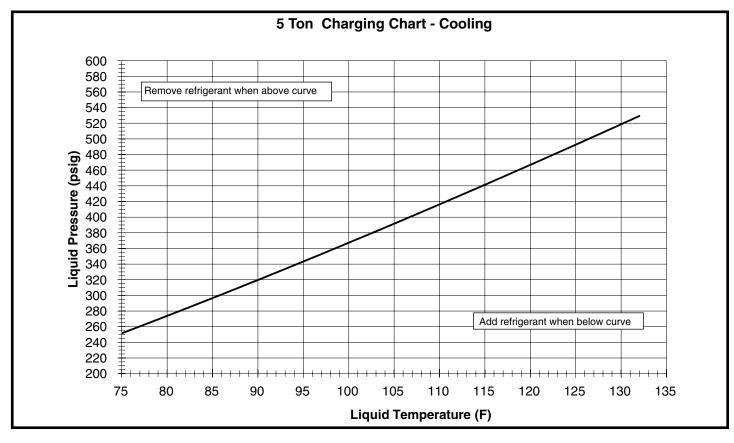
Figure 13. Charging Chart for 5 Ton Models
