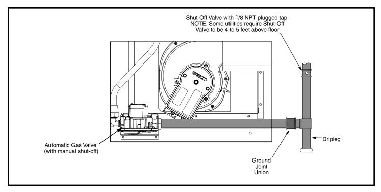
Figure 7. Typical Gas Hookup - Right Side Entry
