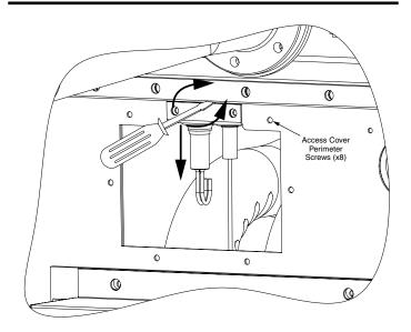
Figure 9. Ignitor Flame Sensor Bracket
