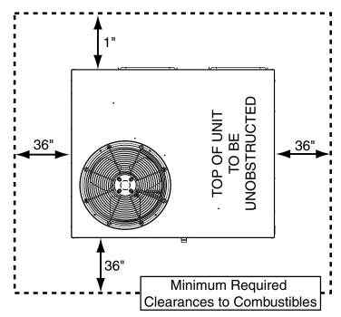
Figure 1. Clearance Requirements
