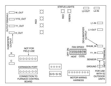
Figure 30. Two-Stage Variable Speed Motor Control Board
