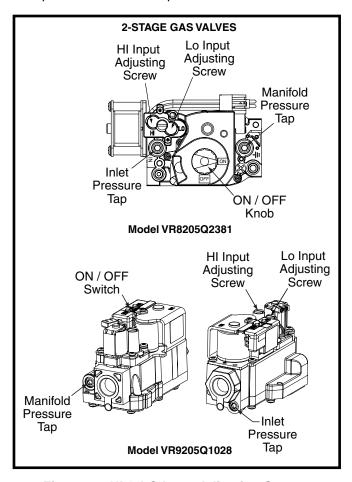
Figure 27. HI & LO Input Adjusting Screws
