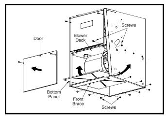
Figure 19. Alternate Removal Method
