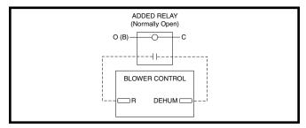
Figure 26. DEHUM Wiring Configuration without Humidistat
