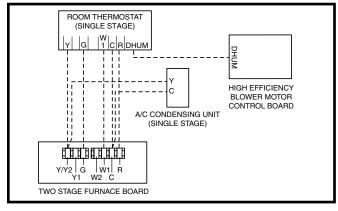
Figure 22. Wiring Configuration 1
