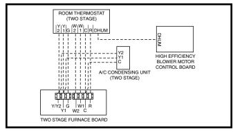
Figure 24. Wiring Configuration 3
