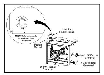
Figure 16. Finish Flange & Rubber Grommets
