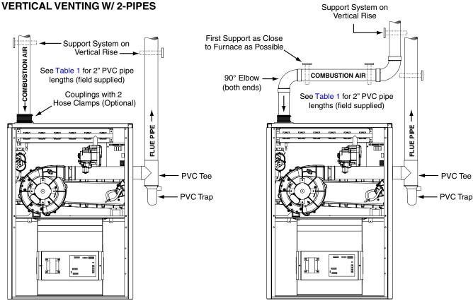
Figure 36. Horizontal & Vertical Venting
