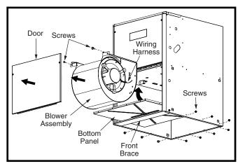
Figure 18. Bottom Panel Removal
