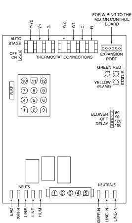
Figure 31. Two-Stage Furnace Control Board
