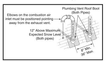
Figure 10. Vertical Vent Termination
