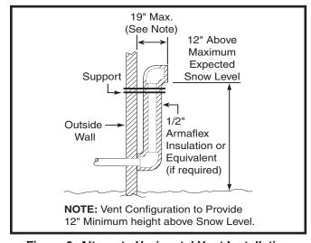
Figure 9. Alternate Horizontal Vent Installation
