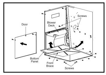
Figure 19. Alternate Removal Method
