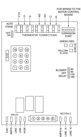
Figure 31. Two-Stage Furnace Control Board
