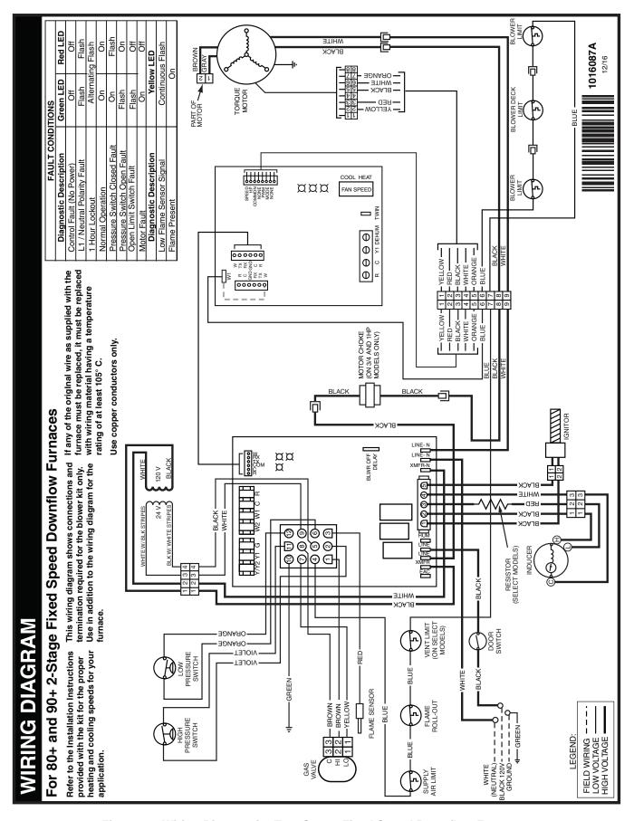
Figure 33. Wiring Diagram for Two-Stage, Fixed Speed Downflow Furnaces
