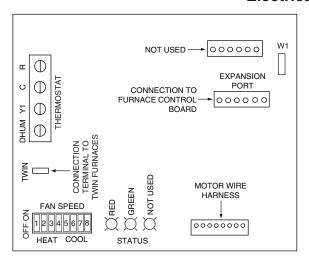
Figure 29. Two-Stage Fixed Speed Motor Control Board
