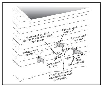
Figure 7. Inlet & Exhaust Pipe Clearances
