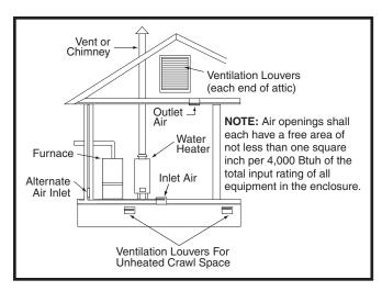
Figure 3. Combustion Air Drawn from a Crawl Space or Vented Attic
