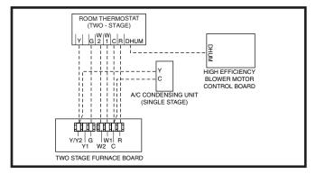
Figure 23. Wiring Configuration 2
