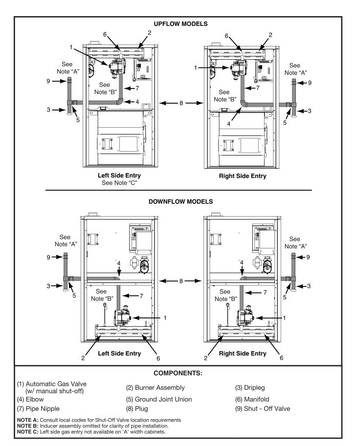
Figure 20. Typical Gas Connections
