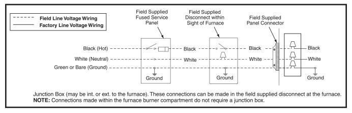
Figure 21. Line Voltage Field Wiring
