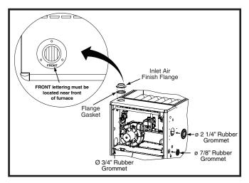
Figure 16. Finish Flange & Rubber Grommets
