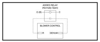
Figure 26. DEHUM Wiring Configuration without Humidistat
