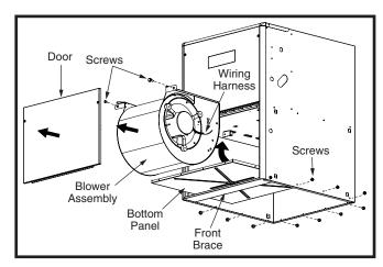
Figure 18. Bottom Panel Removal
