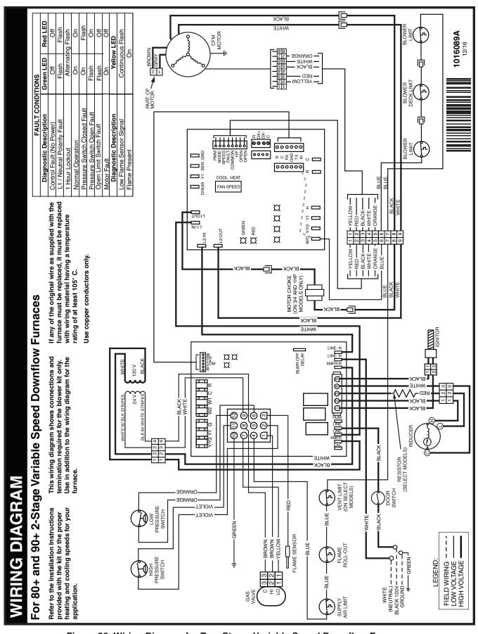
Figure 36. Wiring Diagram for Two-Stage, Variable Speed Downflow Furnaces
