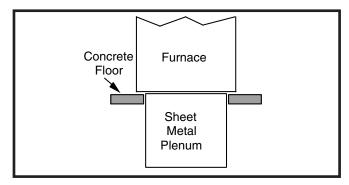
Figure 11. Furnace on a Concrete Slab
