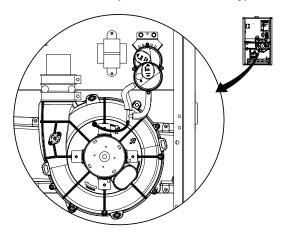
Figure 15. Pressure Switch Tubing for \*TN Downflow Furnaces
