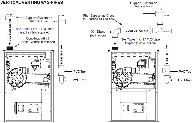
Figure 37. Horizontal & Vertical Venting
