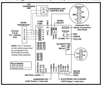
Figure 13. Low Voltage Connections
