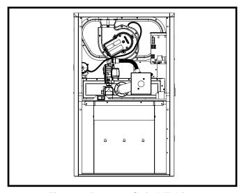
Figure 9. Pressure Switch Tubing
