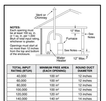
Figure 2. Combustion Air Drawn from Inside
