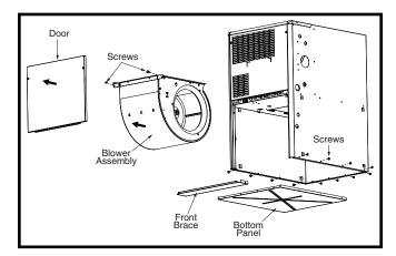
Figure 10. Bottom Panel Removal
