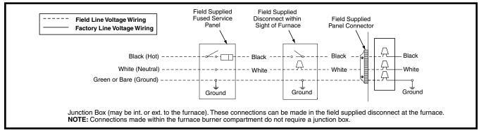
Figure 14. Line Voltage Field Wiring
