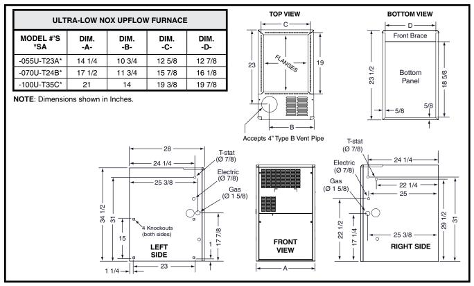
Figure 18. Furnace Dimensions
