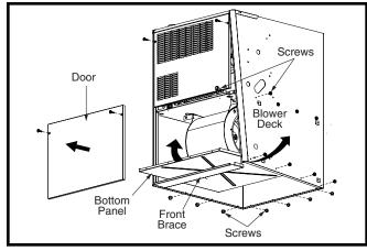
Figure 11. Alternate Removal Method
