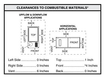
$\uparrow$ Allow 24 in. minimum clearance for servicing. Recommended clearance is 36 in.
