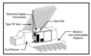
Figure 7. Horizontally Installed on a Platform
