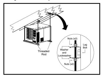
Figure 8. Horizontally Suspended in Attic
