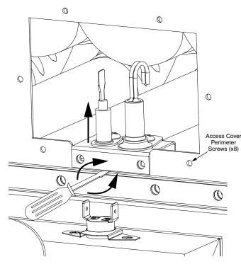
Figure 16. Ignitor Flame Sensor Bracket
