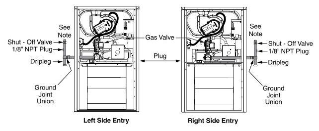
**NOTE:** Some utilities require Shut- Off Valve to be 4 - 5 feet above floor.
