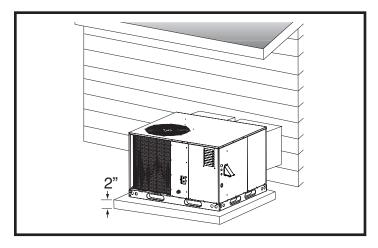
Figure 4. Ground Level Installation
