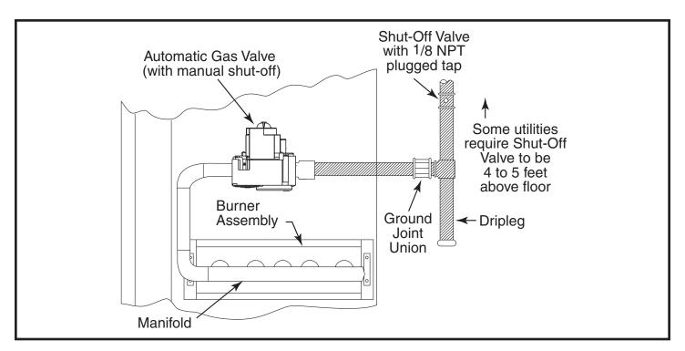
Figure 7. Typical Gas Hookup - Right Side Entry
