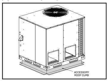
Figure 3. Roof Top Installation
