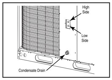
Figure 5. Refrigerant Service Ports & Condensate Drain Locations
