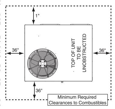
Figure 1. Clearance Requirements
