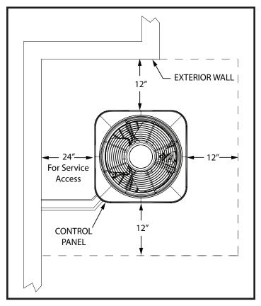
Figure 1. Unit Envelope Dimensions
