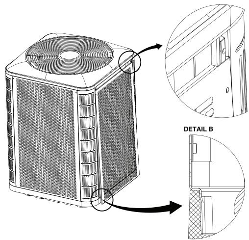
Figure 3. Panel Installation
